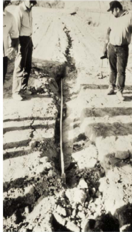
Figure 11-2 Tear in HDPE geomembrane liner system, Canyon C, Chiquita Canyon Landfill (photo courtesy of Calif. EPA, Integrated Waste Management Board)
