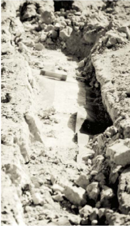
Figure 11-2 Tear in HDPE geomembrane liner system, Canyon C, Chiquita Canyon Landfill (photo courtesy of Calif. EPA, Integrated Waste Management Board)
