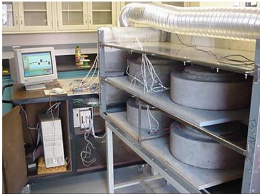
Figure 2.4.1.1. Experimental setup of shrinkage test and recording strain gauge results
