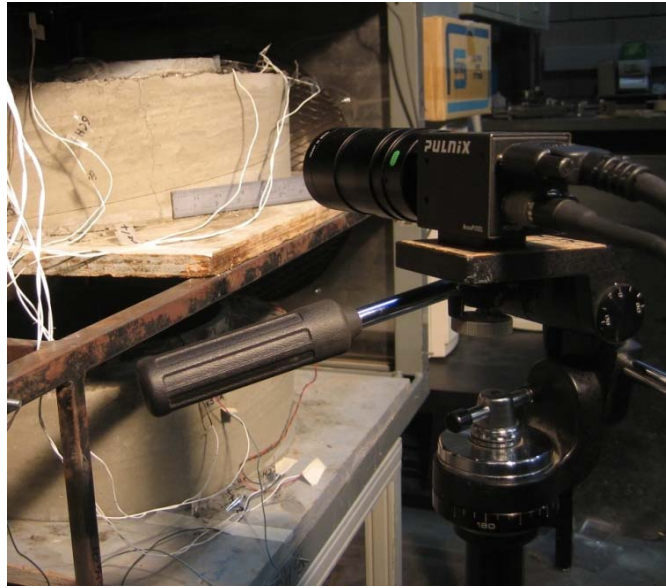
Figure 2.4.3.1. Imaging with the digital camera for crack investigations
