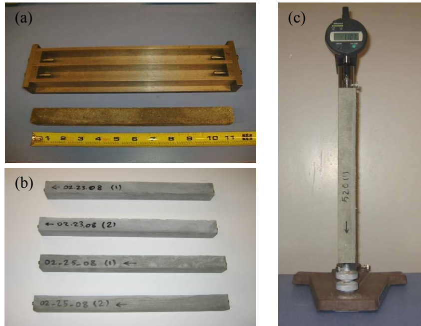
Figure 1.3.1.1. Molds, samples and digital comparator dial used in free shrinkage tests
