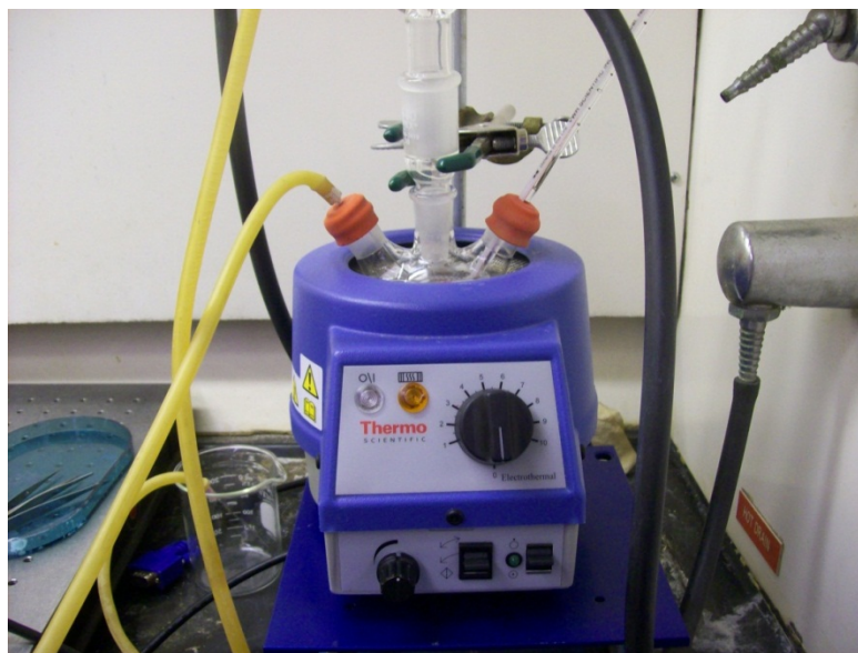
Figure 4. Nanoparticle polymerization. The valve on the left connects to a nitrogen tank, while the temperature is monitored using the thermometer on the right. The condenser ensures the solvent does not boil off.
