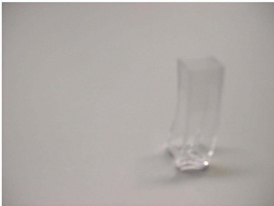
Figure 28. Warped cuvette after experiencing glass-transition temperatures
