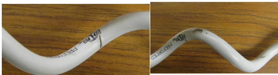
Figure. 37 Damper sample showing damage in the outer sheath
