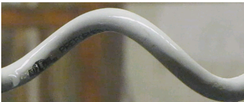
Figure. 44 Surface of the damper when 15 kV is applied
