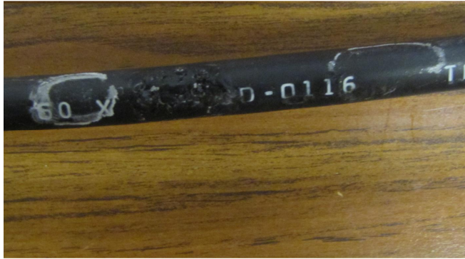
Figure. 35 Cable sample showing damaged outer sheath
