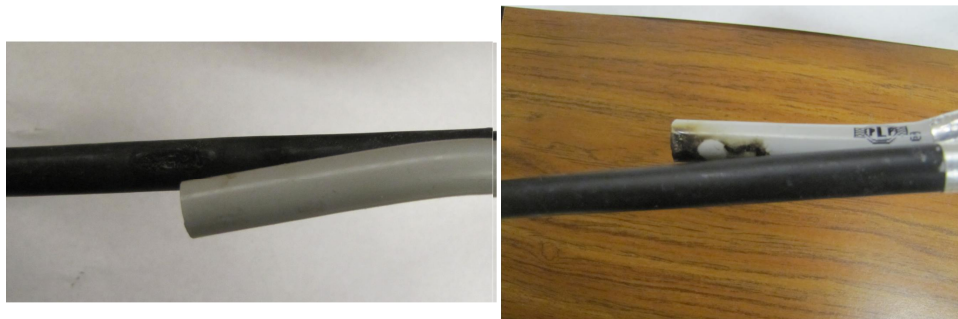
Figure. 35 Cable sample showing damaged outer sheath
