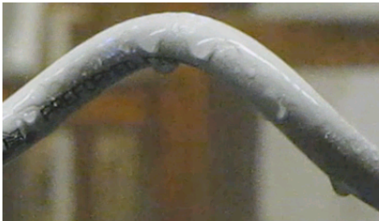
Figure. 43 Surface of the damper when 10 kV is applied
