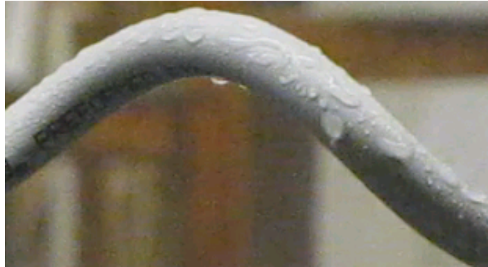
Figure. 42 Surface of the damper at 5 kV with water droplets on the surface
