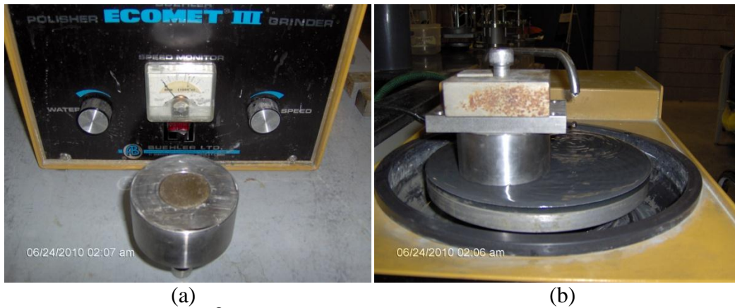
FIG. 3.16. (a). Buehler ® Ecomet III Manual Grinder and Grinding/Polishing Jig. (b). Grinding/Polishing Jig Loaded with Weights During Manual Grinding Process.
