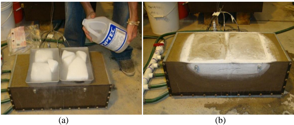
FIG. 3.9. (a) Freezing of Fully Saturated Ottawa 20/30 Sand. (b) Resulting Semi-circular Mass of Stabilized, Frozen Soil.
