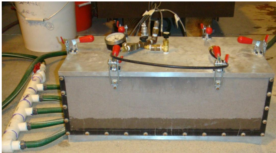
FIG. 3.8. The Box Used for Wet Sample Preparation during Saturation Process.
