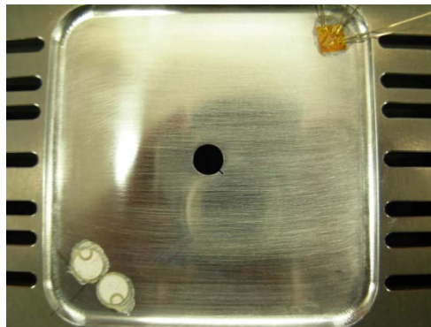
Figure 4.23 Cruciform specimen with a 45o notch at the center hole for fatigue test
