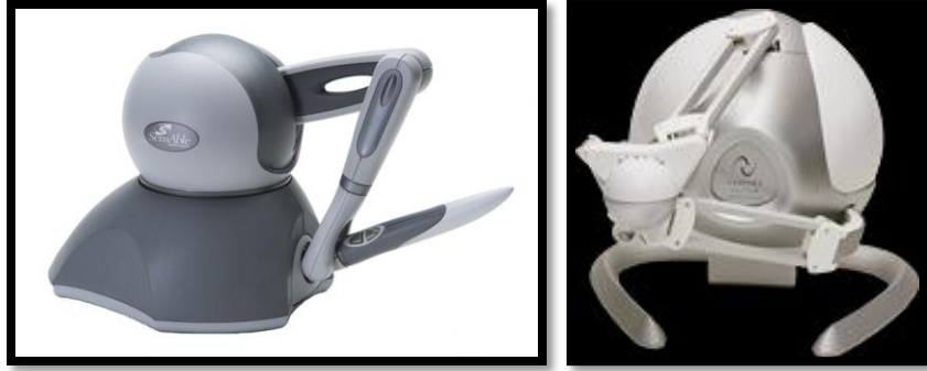
Figure 6. The PHANTOM® (left) and the Falcon® (right) are both force feedback devices used to exert forces upon the human hand to simulate the shape, texture and/or material of virtual objects. The PHANTOM® is more commonly used as a research tool, whereas the Falcon® is designed for gaming.
