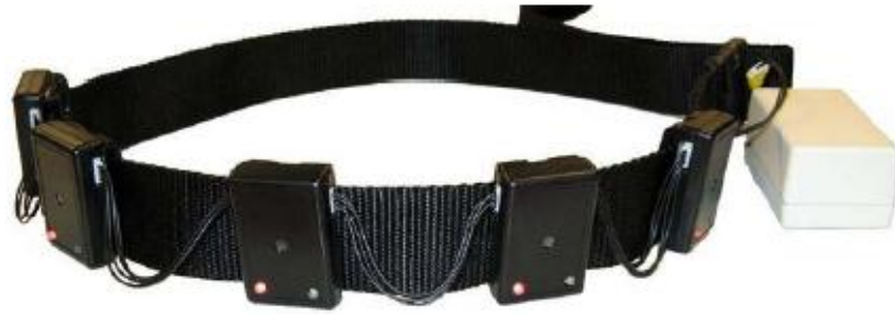
Figure 18. The haptic belt that was used in this study [68]. The tactor modules (the black boxes) each contain a vibration motor, and are connected through an I 2 C bus. The main controller (the white box) is also shown.
