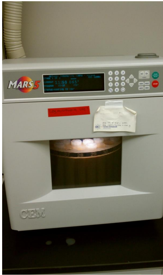
Figure D.3. MARS Express microwave digester.
