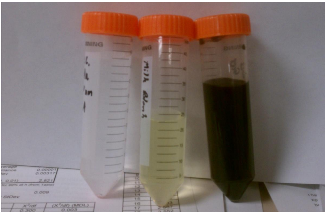
Figure 3.1. Whole milk digested by hot plate digestion (right), microwave digestion (center), and microwave digestion with hydrogen peroxide (left). All samples shown were blanks, with no \text{TiO}_2 added.
