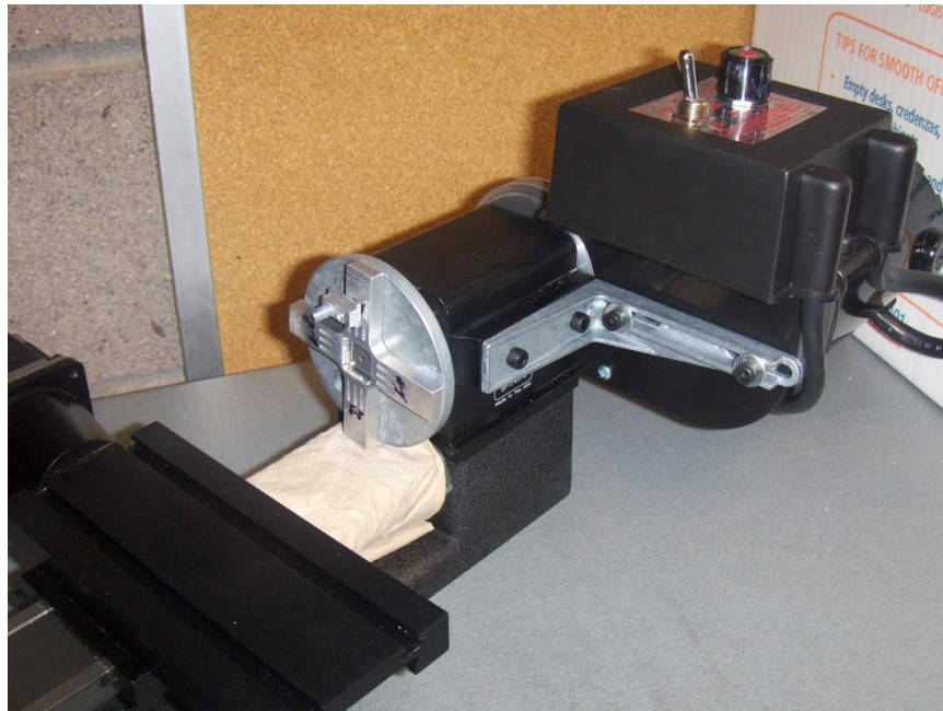
Figure 3.10: Picture showing the cruciform fixtured in the lathe.
