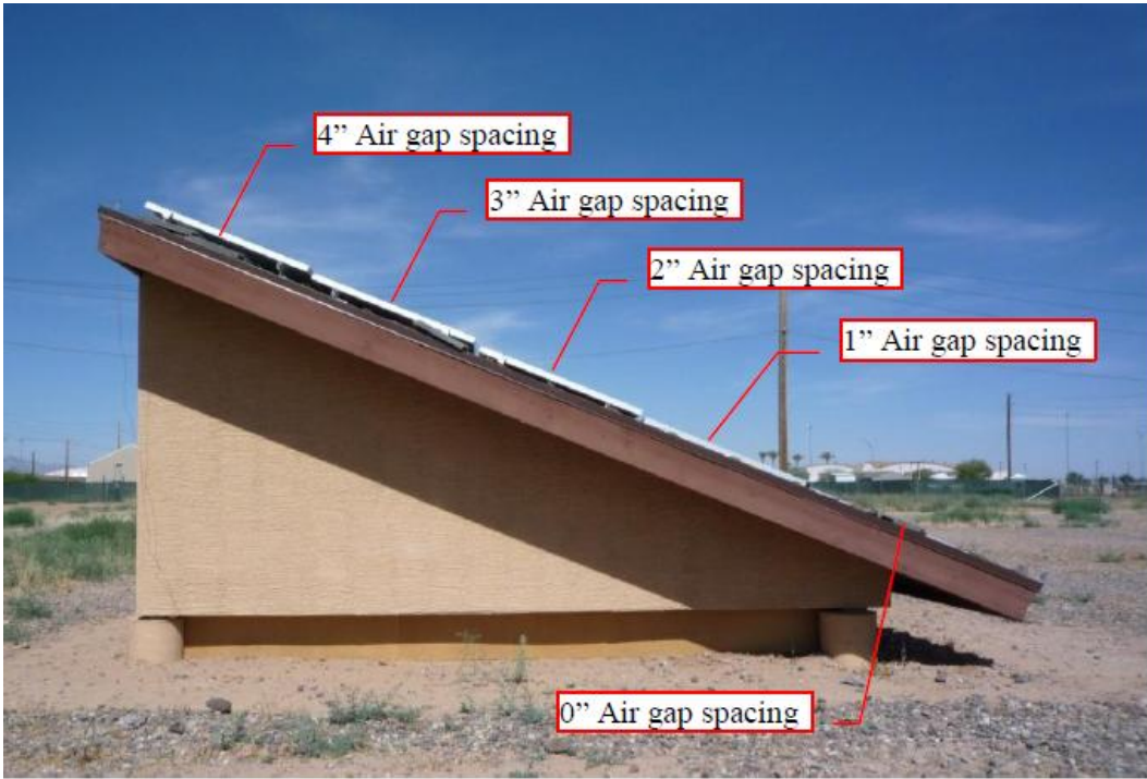
Figure 13 Side view of the simulated rooftop structure with installed modules[3]
