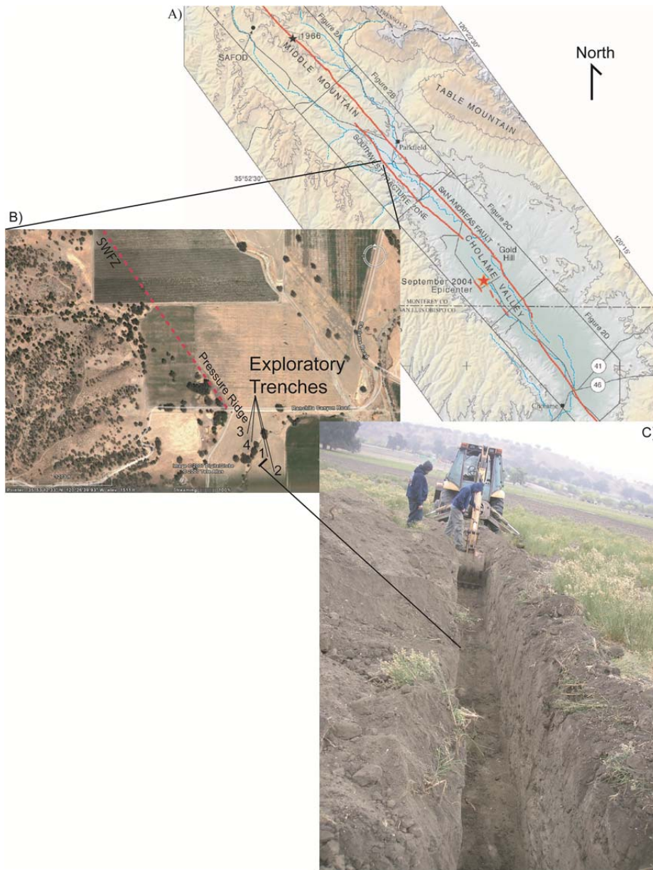
Figure B1. A) The Southwest Fracture Zone (SWFZ) is parallel and about 1 km SW of the main SAF along the Parkfield segment (map from Rymer et al., 2006). B) The SWFZ exploratory paleoseismic trenches (black footprint and sites 1-4) were located just south of Ranchita Canyon Road to the sides of an ephemeral stream incised into an alluvial fan extending from Ranchita Canyon. This area of
