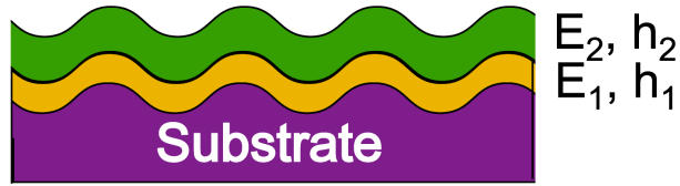
Figure 1.4 Schematic of mechanical induced two-plate wrinkling. The PDMS is pre-strained 2-5% followed by the integration of two thin films. Wrinkling is induced by compressing the pre-strained system.
