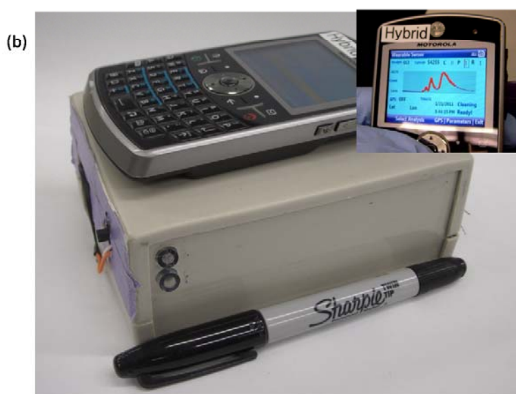
Fig. 1. (a) Schematic representation of the hybrid device. (b) The picture of the hybrid device, insert: the smartphone user interface showing a real time detection of a BTEX mixture sample.
