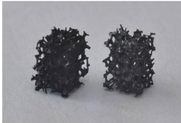
Figure 18. Sponge-type carrier before (left) and after (right) TiO 2 coating by the O method. The color of sponge-type carrier originally was black, but it changed to grey due to TiO 2 coated on the outer surface.
