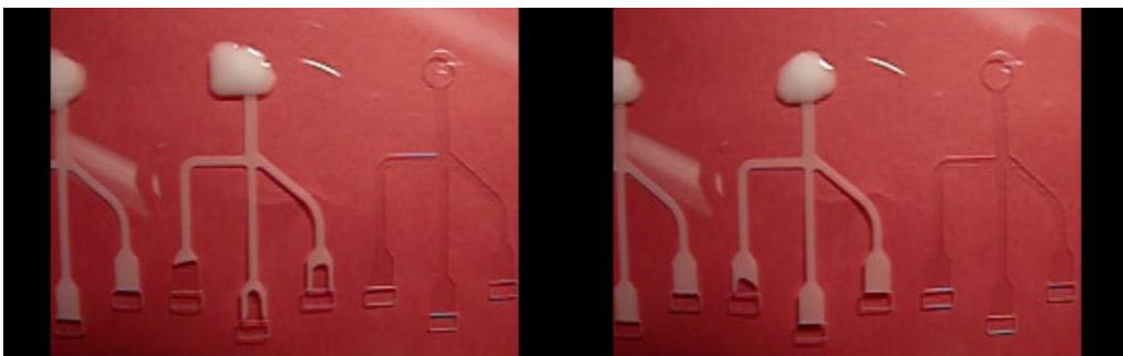
Defects observed in Hydraulic press using water based dye and whole milk as fluid.
