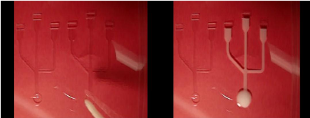
Fig: Shows a ballistic press three channel with whole milk as the fluid. Images show before the fluid was introduced into the channel and after the flow is completed in the channel.
