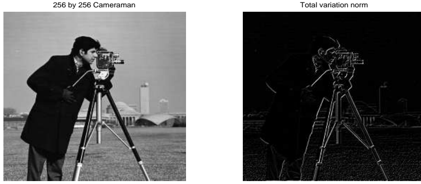
Figure 2.1: From left: (1) The 256 by 256 Cameraman; (2) The Isotropic total variation norm of the 'Cameraman'.
