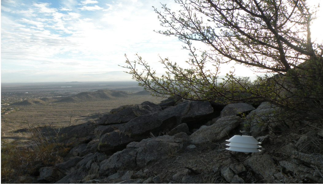
Figure 10. Hobo data logger inside a solar radiation shield at South Mountain Municipal Park, January to March 2010.
