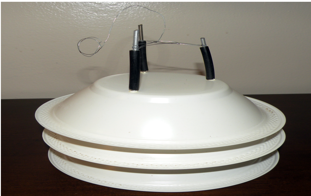
Figure 8. Solar radiation shield for Hobo data loggers used in South Mountain Municipal Park, January to March, 2010.
