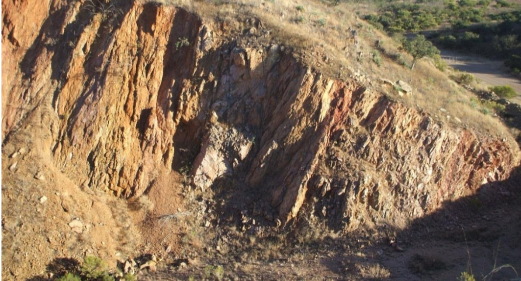
Figure 2-25 Bedding-parallel structure that hosted mineralization within Ruben Pit, looking southeast. The beds strike northwest, dip northeast and are overturned. Mineralization was sited at the intersection of the northwest-trending reddish oxide zones and a northeast structure, now the long axis of the pit (from left to right).
