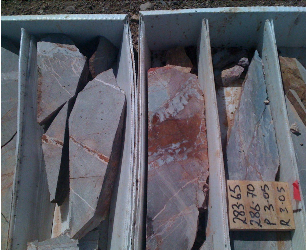
Figure 2-71 Drill core from ARTG-001, 280 m, with oxidation of quartz + sulfides crosscutting older cleavage.
