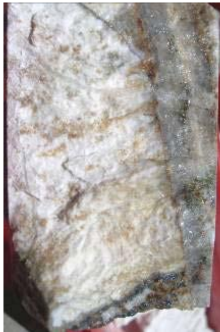
Figure 3-14 Core photo of drill-hole SE-15-5, Teck Cominco, from San Enrique reveals wollastonite-garnet skarn with quartz/chalcopyrite/moly veins postdating the formation of skarn.
