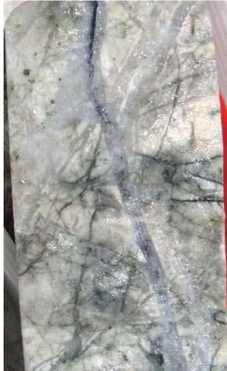
Figure 2-64 Quartz stockwork in potassium-altered hornfels. Note the late, nearly core parallel vein with axial molybdenite. Core from EN-001, depth unknown. (Teck Cominco, 2006).
