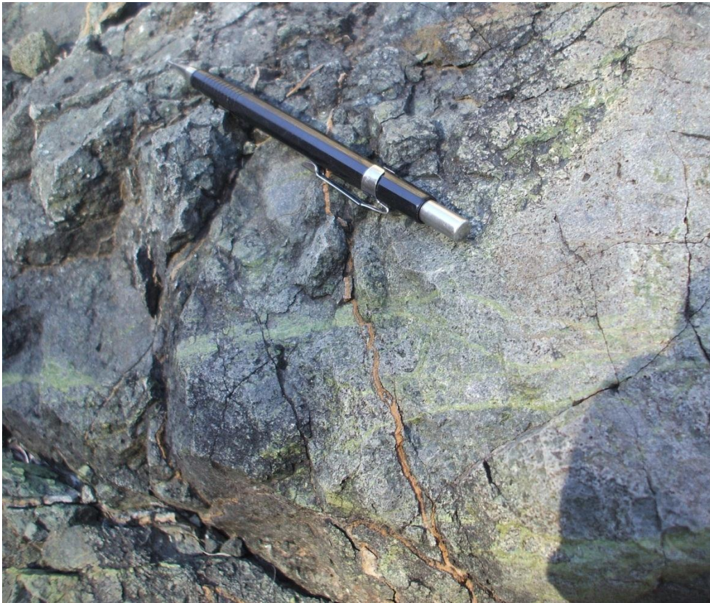
Figure 2-12 Disseminated and fracture chlorite in diorite, cut by late-stage calcite stained with hematite.
