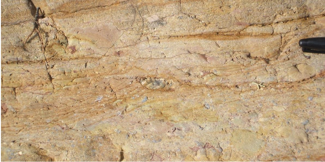
Figure 2-2 Stratigraphic tops were determined using graded beds, crossbeds and other sedimentological indicators. Top is up in this photo. Graded beds and crossbeds in the Ksl. Tops were important for determining structural overturning present in the Animas 2009 deep drilling.
