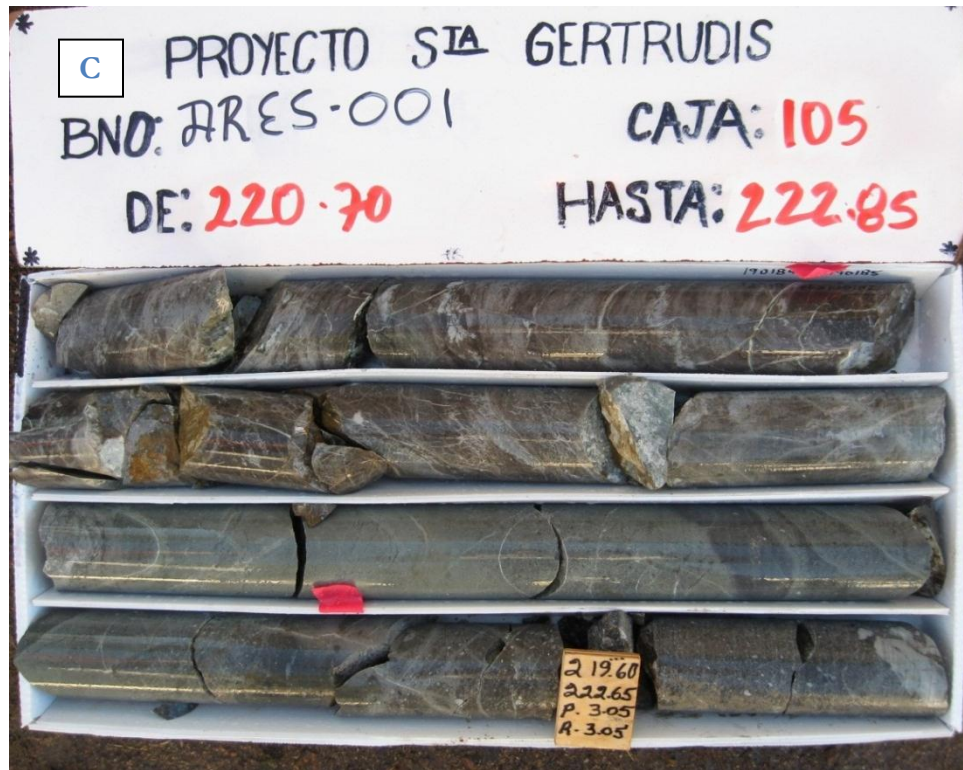
Figure 2-5 6.50 m of core from ARES-001 showing lower gradational contact between interbedded, basal oyster-bearing limestones of the Morita Formation (Figure A and B) grading into greenish sandstones and pea-sized, pebble conglomerate (Figure C) of the Morita Formation. Calc-silicates between the limestone and sandstone (top of Figure C) are strong, brown-biotite hornfels. Core length is 2.4 m per box.
