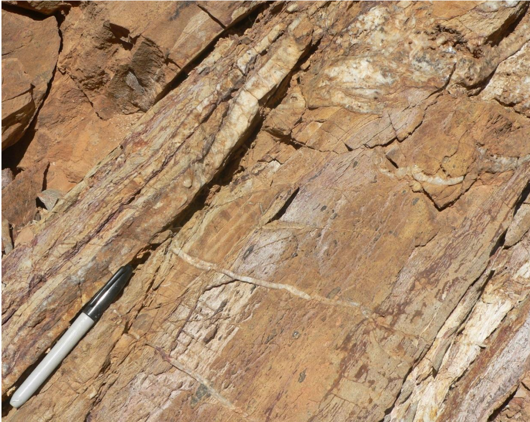
Figure 2-70 Bedding-parallel shear (pen is parallel to bedding) and quartz veins associated with hematite, goethite, argillization and color leaching. Note that shear in the upper right is localized at the change in rock strength at the sandstone/siltstone interface and crosscuts an older vein set. Photo from Gregorio Mine, courtesy of S.J. Reynolds.
