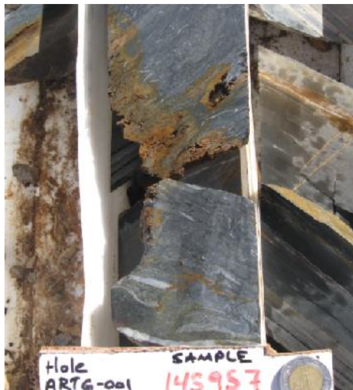
Figure 2-57 Initial decalcification of Ko limestone along front, with bedding plane control. A Centavo coin for scale.
