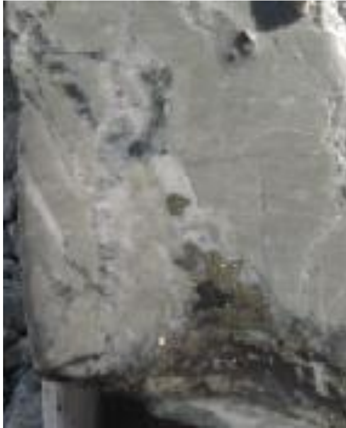
Figure 2-68 Pyrite and sphalerite in a highly altered felsic dike from 2009, Main District, Animas drilling program. Core from ARTG-001, 474.15 m. Sample assayed at 6.3 ppm Ag, 210 ppm Ba, 39.2 ppm Cd, 1020 ppm Pb and 1715 ppm Zn.
