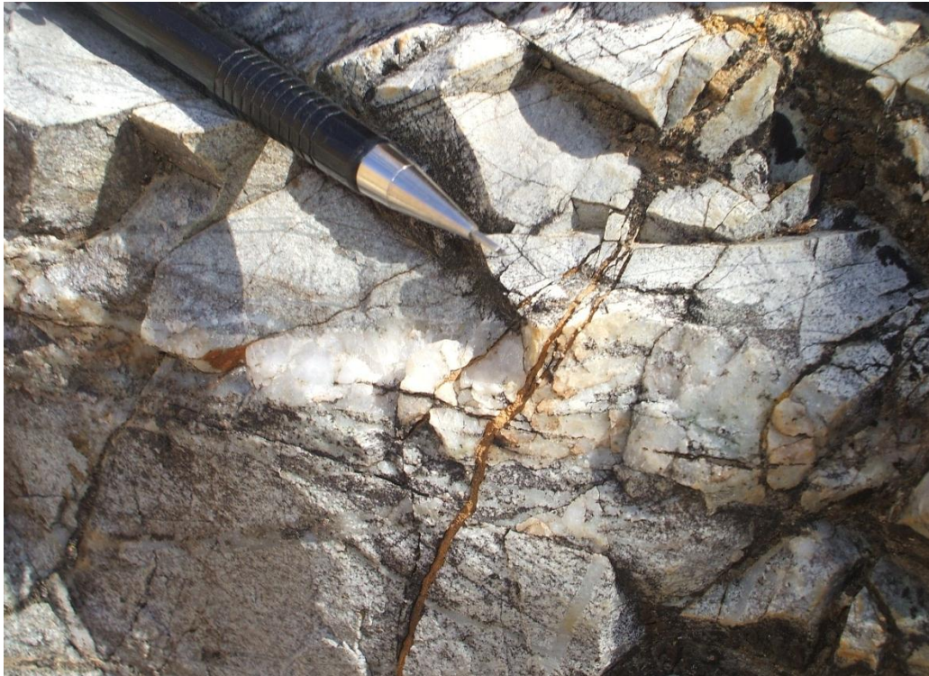
Figure 3-28 Enedina hornfels and quartzite cut by high temperature quartz vein, all of which are then cut by the now-oxidized sulfide veinlets.
