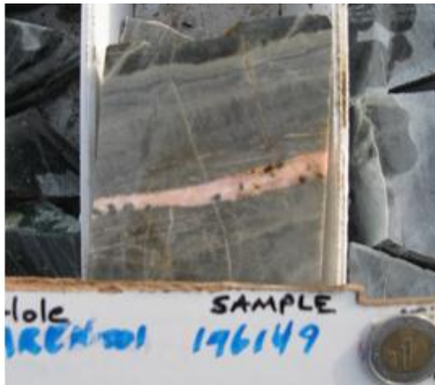
Figure 2-63 Rhodocrosite + pyrite that rapidly oxidized within minutes of cutting. A Centavo coin for scale. Core from AREN-001.
