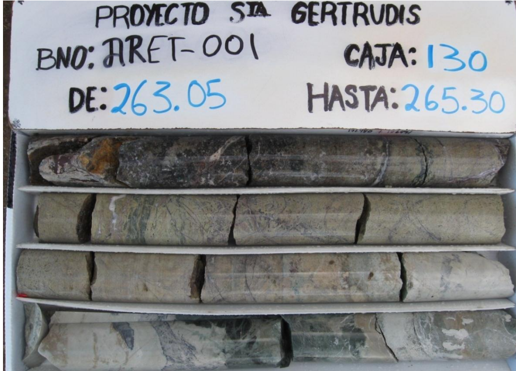
Figure 3-17 2.40 m of core from ARET-001, El Tigre with gradation from pyroxene hornfels in upper left grading to magnetite skarn then grading to andradite garnet skarn in the middle two rows, and marble as pure white at end of third row and most of fourth row.
