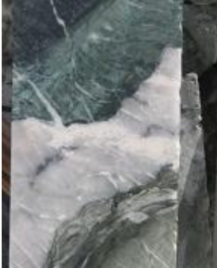
Figure 2-67 Quartz + feldspar + molybdenite cutting chlorite/epidote alteration. Core from AREN-001, 356 m depth. A Centavo coin for scale. (Animas, 2009)
