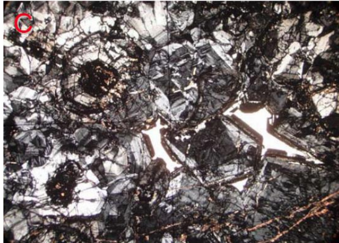
Figure 3-15 ARET-001, 277 m. Zoned andradite garnet skarn (A) shows light brown equant garnet with colorless calcite in PP light, 5.7 mm wide. (B and C) show the garnet in XP, with anomalous birefringence (Burnham Petrographics, 2009).
