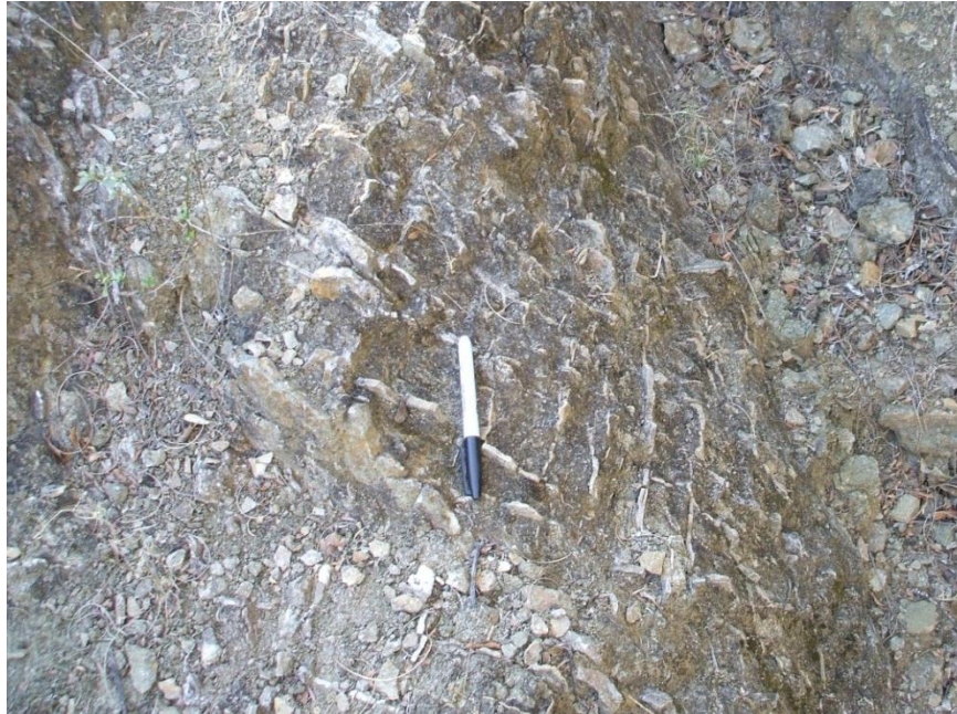
Figure 2-47 Ladder calcite veins cutting diorite and disseminated Cu-oxides. South of Dora.
