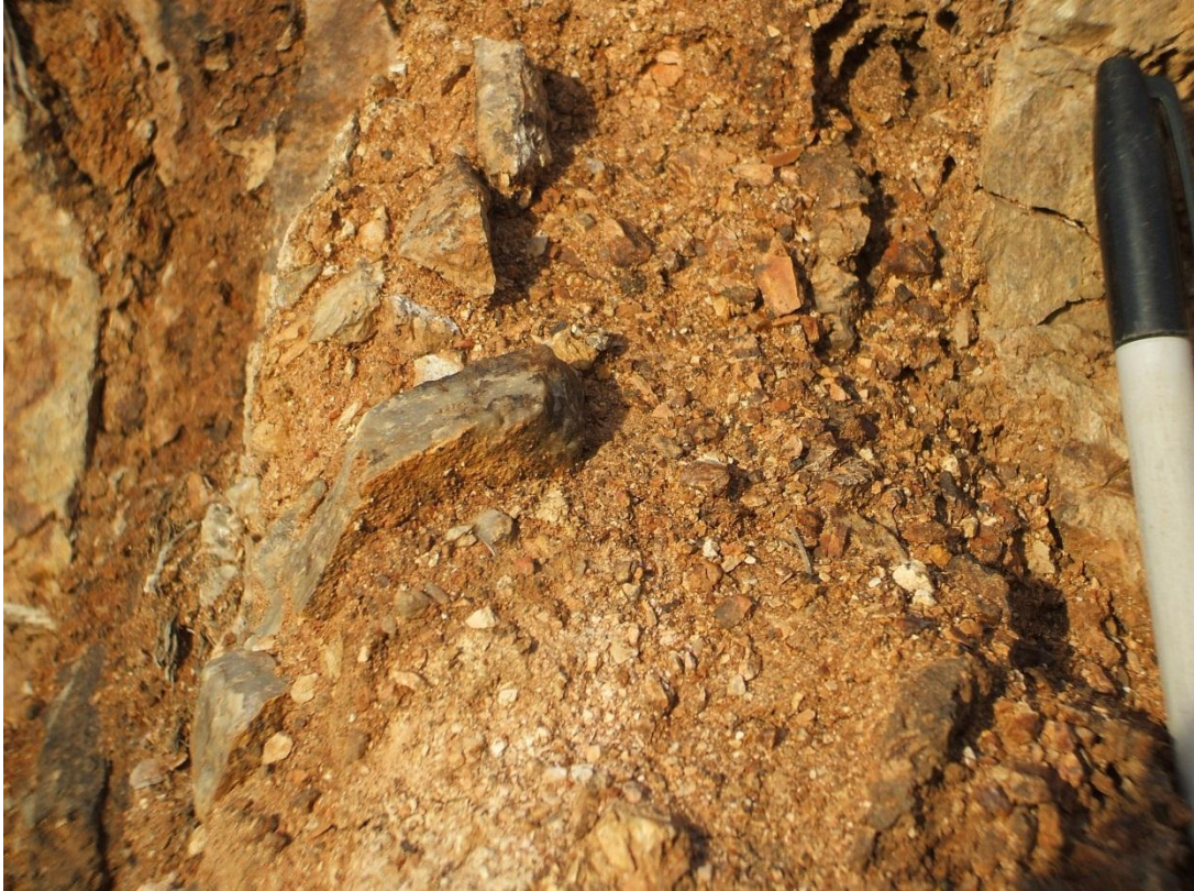
Figure 2-69 Quartz vein fragments in fault breccia in Dora Pit. These fragments can contain gold, or can be barren.
