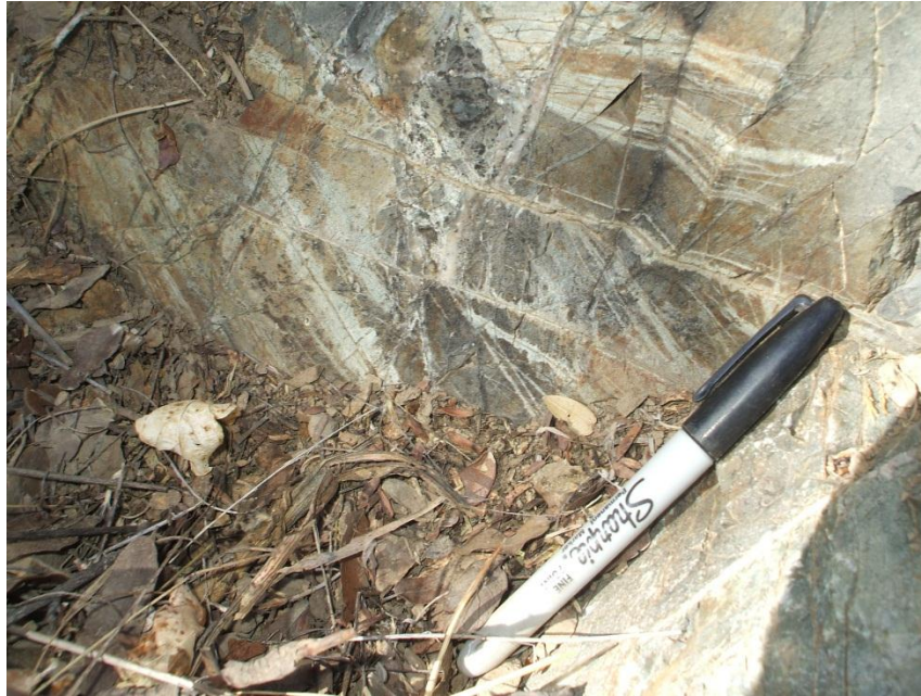
Photo 3-7 Distal alteration of brown-biotite hornfels northwest of El Tigre similar to drill core from Mirador and El Tigre. Note albite-epidote hornfels alteration along fractures.
