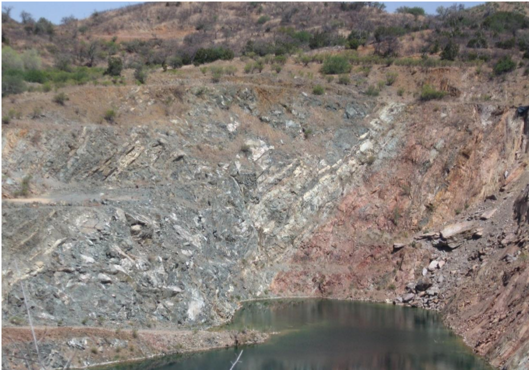
Figure 3-45 View looking 330° at Becerros Norte. At left, dark grayish green rock is pre-mineral diorite with hornfels associated with local, contact metamorphism. Reddish area on right is the mineralized shear-zone that was the primary mined ore zone.
