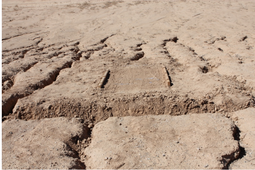
Figure A5: A Test Plot Surrounded by Ditches to Divert Rain Water
