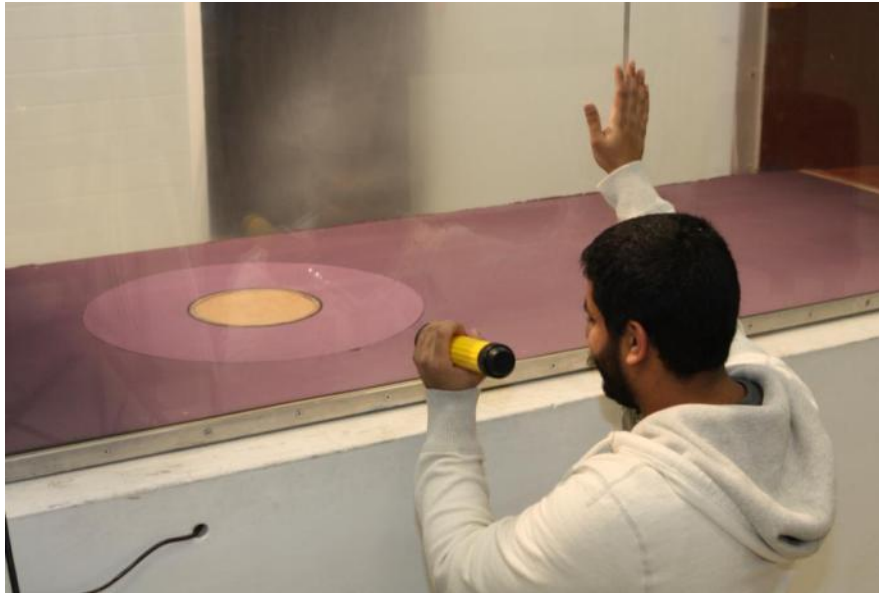
Figure 28: Observing Threshold Friction Velocities.
