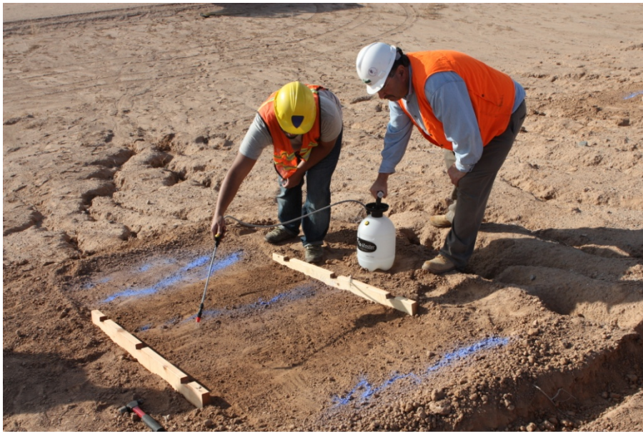
Figure A2: Applying Biopolymer Mixtures
