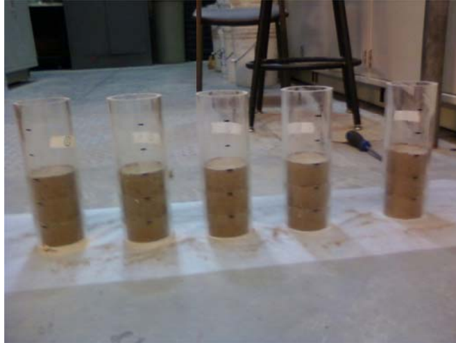
Figure 4.30: Sample Set-up and Compaction of Dry Section.
