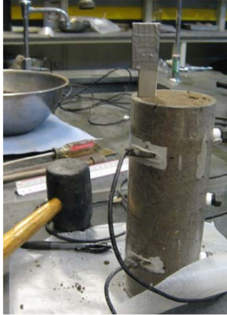
Figure 4.116: Creating Crack Formation for Test No. 6 C (1).
