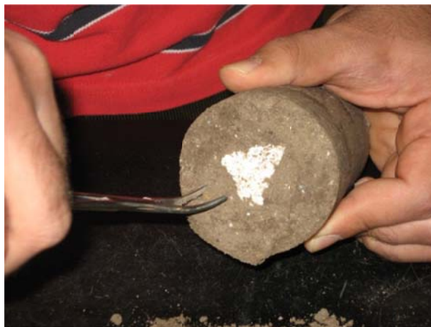
Figure 4.34: Obtaining Filter Paper Sandwich from Soil Sample.
