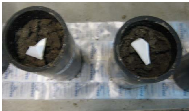
Figure 4.63: Test No. 4 Filter Paper Sandwich Placement and Soil Scarification.
