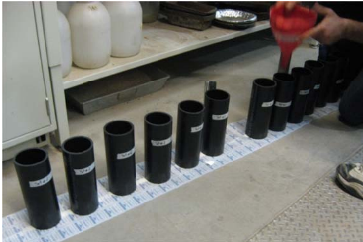
Figure 4.62: Test No. 4 Sample Compaction.
