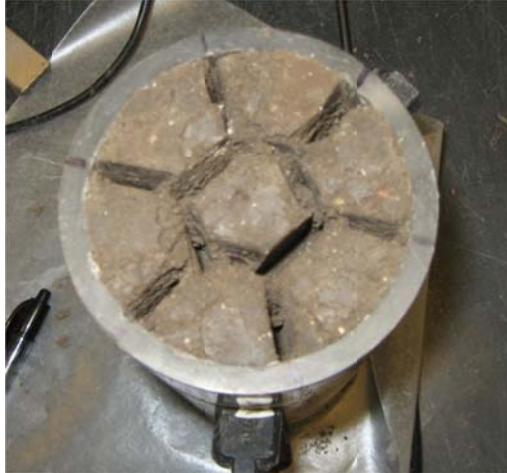
Figure 4.119: Creating Crack Formation for Test No. 6 C (4).
