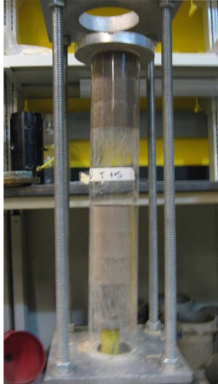
Figure 4.94: Test No. 5 Sample Creation Extruding Process.
