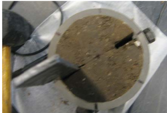
Figure 4.117: Creating Crack Formation for Test No. 6 C (2).
