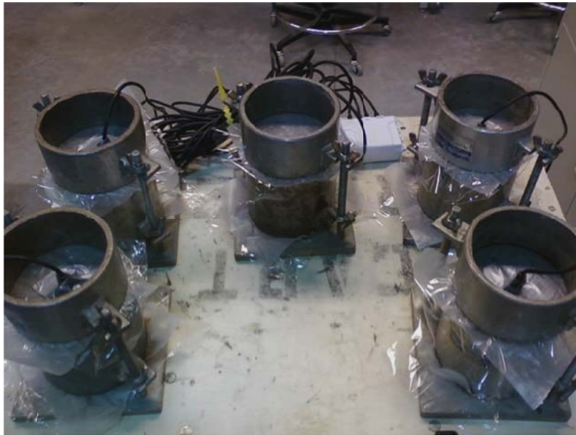
Figure 4.9: Volumetric Probe Calibration.
