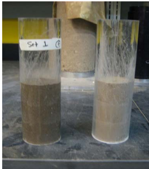
Figure 4.92: Test No. 5 Soil Sections Compacted in Sample Tubes.
