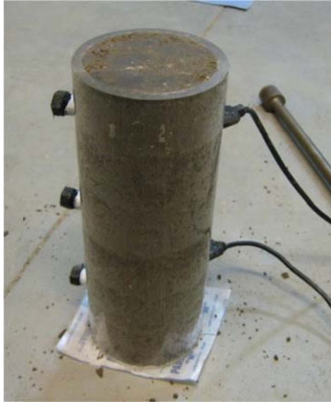
Figure 4.44: Test No. 6 I Compacted Sample with Vol. Probes Installed.
