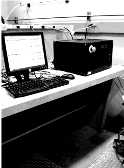
Figure 3.2. Computer and digital signal conditioning and control device used during testing.
