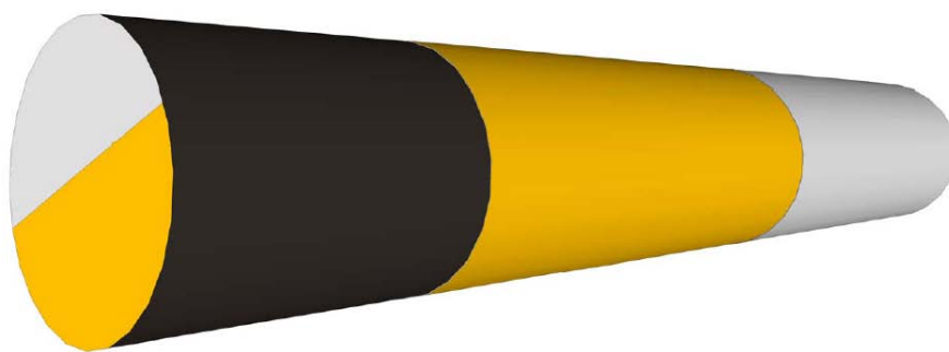
Figure 11: Conceptual design for a gold-platinum nanomotor that would undergo chemotaxis in a hydrogen-peroxide concentration gradient, the black segment is non-conducting.
