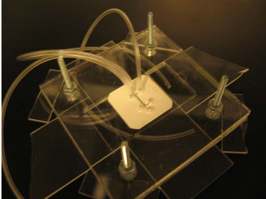
Figure 32: Initial channel structure design. Lower surface is a glass microslide. The structure is sandwiched between two acrylic plates.
