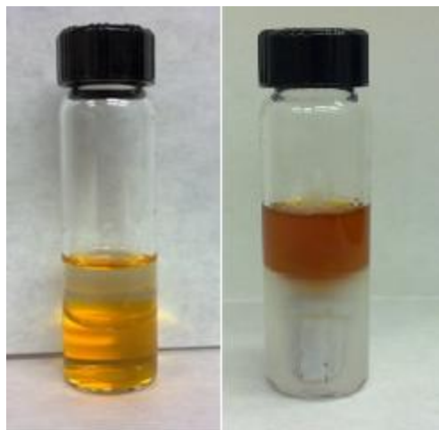
Figure 12 Two-phase transfer processes before and after the transfer (ALS based procedure)
