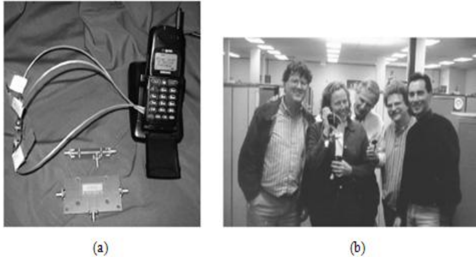
Figure1.3 (a) Image of the first FBAR duplexer and cell phone. A ceramic duplexer is shown in front for size comparison. (b) Members of the FBAR team in 1998 were making the phone call with FBAR duplexer (Ruby 2009).
