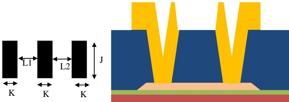
Fig. 4.9 (a) “SDI” Mask (b) Cross-sectional view after contacts isolation
