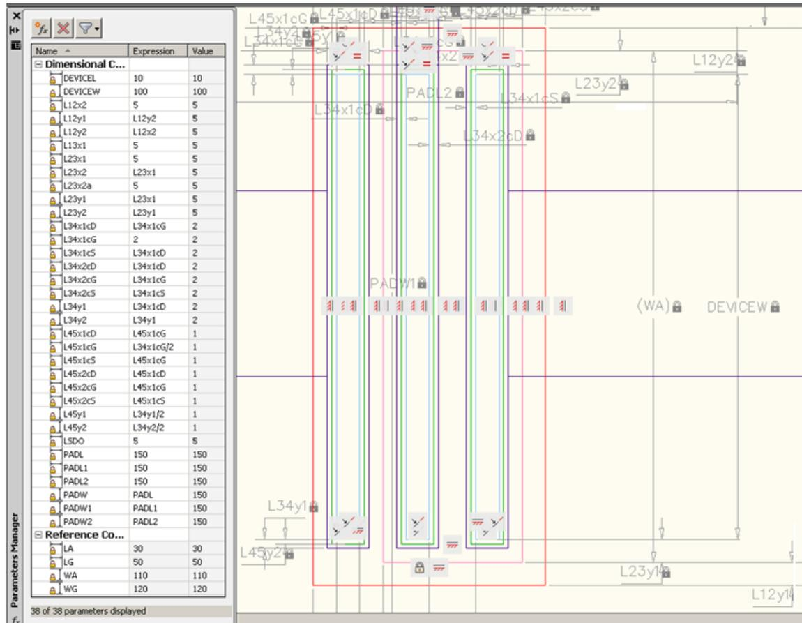
Figure 12.5 AutoCAD Screen shot depicting the MOSFET layers with dimensional constraints
