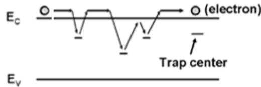
Fig.7.10 (e) Electron trapping and WTA
