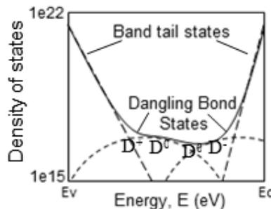
Fig. 3.1 Density of states diagram
