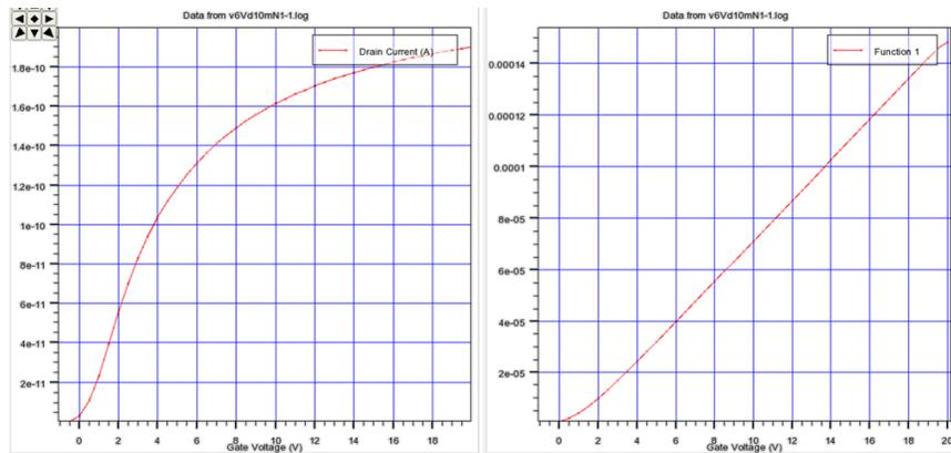
Fig. 9.3 (a)  $I_D$  and (b)  $I_D/\sqrt{g_m}$  versus  $V_{GS}$  plots for  $L = 6 \mu\text{m}$ ,  $V_{DS} = 10 \text{mV}$
