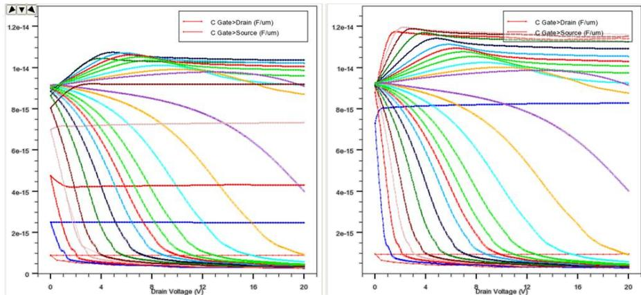
Fig. 8.3  $C_{GS}, C_{GD}$  versus  $V_{DS}$  for  $\mu_n=0.1$  and  $1\text{cm}^2/\text{Vsec}$
