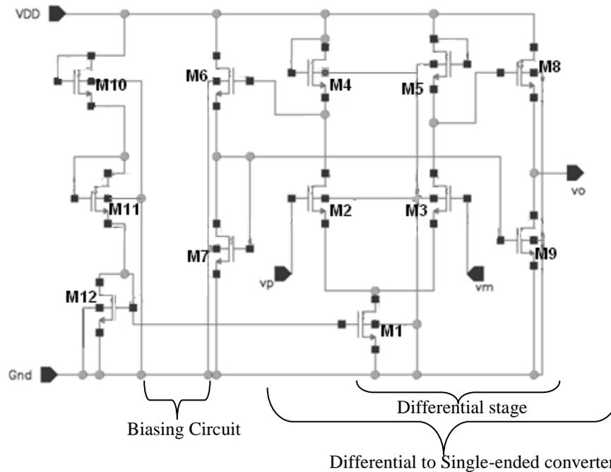
Fig.11.1 Operational amplifier design
