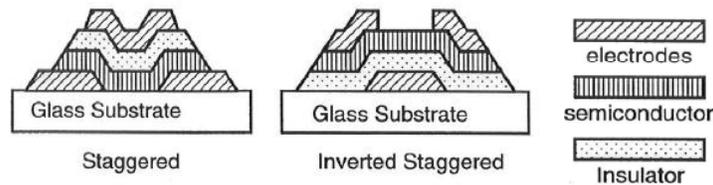
Fig. 3.3 Staggered and Inverted staggered structures
