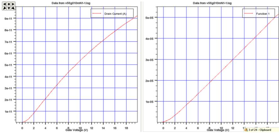
Fig. 9.5 (a)  $I_D$  and (b)  $I_D/\sqrt{g_m}$  versus  $V_{GS}$  plots for  $L=56\ \mu\text{m}$ ,  $V_{DS}=10\ \text{mV}$
