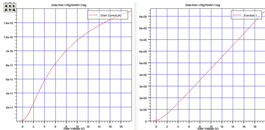
Fig. 9.4 (a)  $I_D$  and (b)  $I_D/\sqrt{g_m}$  versus  $V_{GS}$  plots for  $L = 16 \mu\text{m}$ ,  $V_{DS} = 10 \text{mV}$
