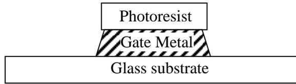
Fig 4.3 Cross-sectional view after etching away metal
