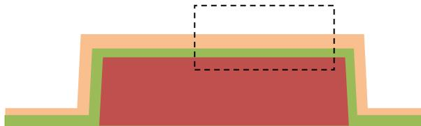
Fig. 4.4 Cross-sectional view after depositing active channel
