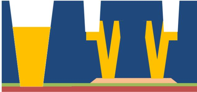
Fig. 4.11 Cross-sectional view after using “CONTACT” mask
