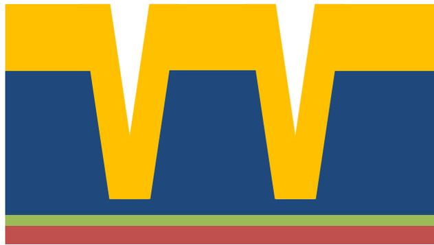
Fig. 4.8 Cross-sectional view after depositing contact a-Si:H
