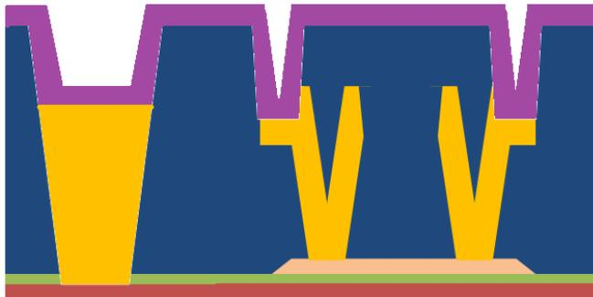
Fig. 4.12 Cross-sectional view after deposition of metal over contact regions
