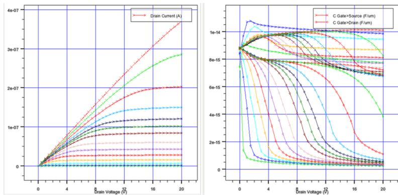
Fig. 9.6 (a)  $I_D$  (b)  $C_{GS}, C_{GD}$  versus  $V_{DS}$  plots
