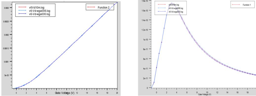
Fig.7.8 (c)  $\sqrt{\frac{I_D}{g_m}} - V_G$  plots with WGA varied (d)  $g_m$  plots with WGA varied
