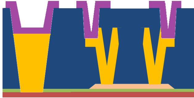
Fig. 4.13 Cross-sectional view after using “METAL” mask
