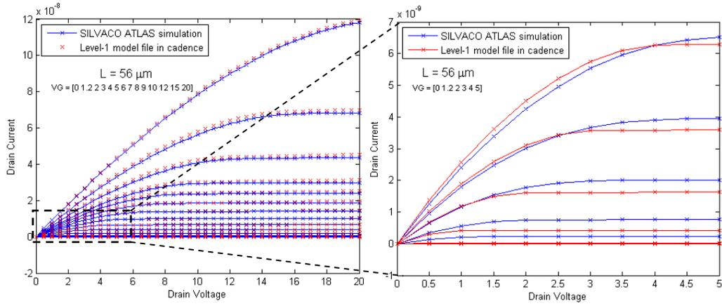
Fig.10.3 Model performance for  $L= 56\mu\text{m}$  (Test conditions specified on the plots)
