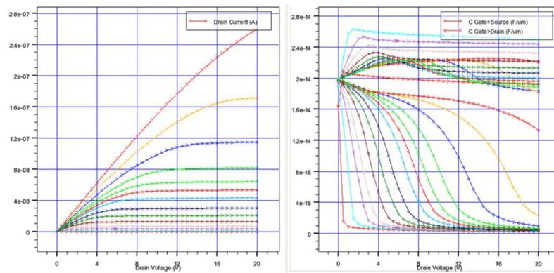
Fig. 9.7 (a)  $I_D$  (b)  $C_{GS}, C_{GD}$  versus  $V_{DS}$  plots
