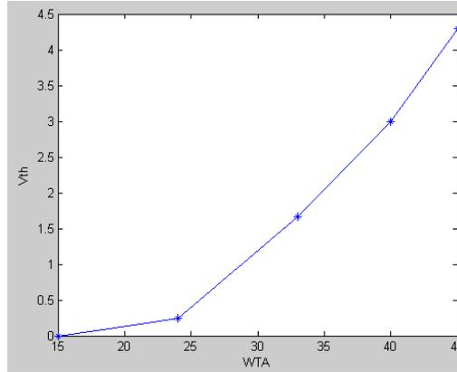
Fig.7.10 (f) Threshold voltage as a function of WTA
