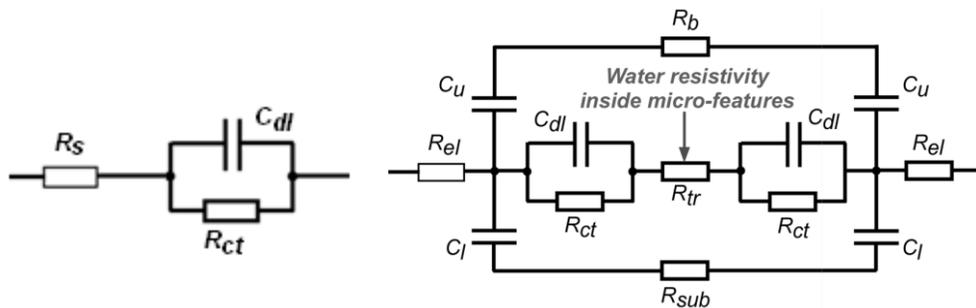
Fig.1.2 (a) The Randles cell (b) Model with all the parasitics included
