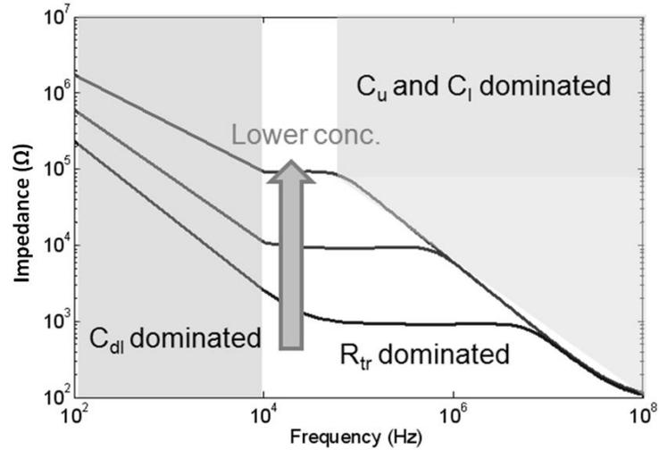
Fig.1.3 ECRS impedance versus frequency
