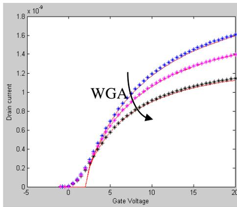
Fig.7.9 (e)  $R_{SD}$  model performance
