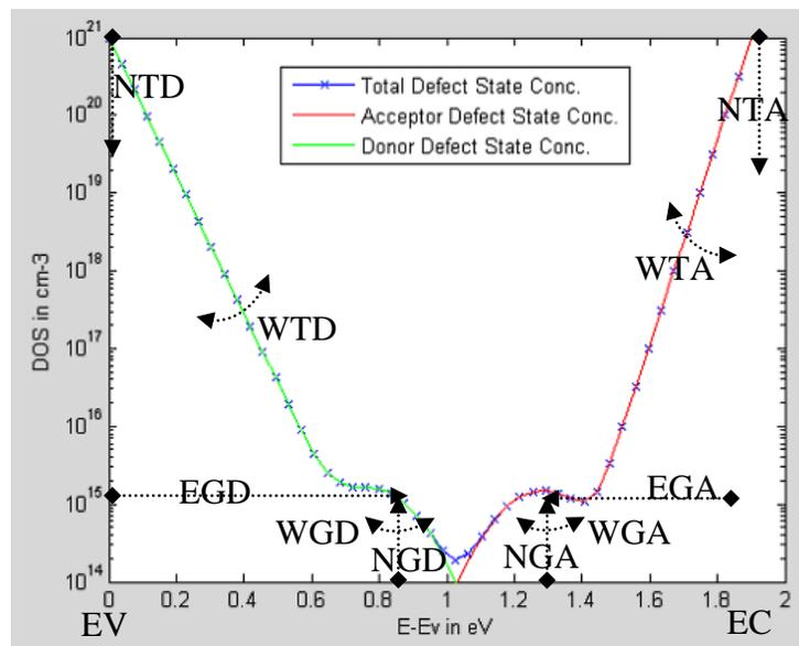
Fig.7.2 Density of states in SILVACO –an example plot
