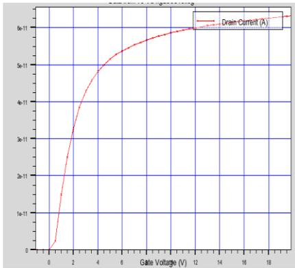
Fig.7.7 (e)  $I_D$  for  $NGA = 9 \times 10^{16} / \text{cm}^3$
