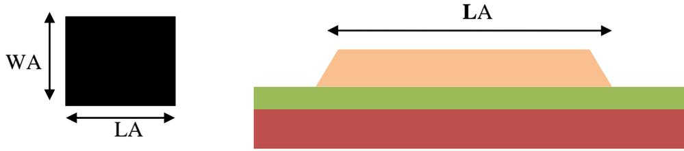
Fig. 4.5 (a) “ACTIVE” Mask (b) Cross-sectional view after patterning active area (Zoomed-in to dotted region in fig.4.3)
