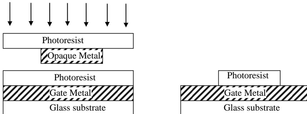
Fig 4.2 Cross-sectional view after etching away photoresist
