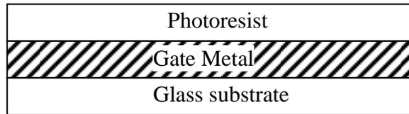
Fig 4.1 Cross-sectional view after applying photoresist
