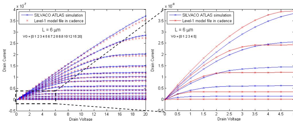
Fig.10.2 Model performance for  $L= 6\mu\text{m}$  (Test conditions specified on the plots)
