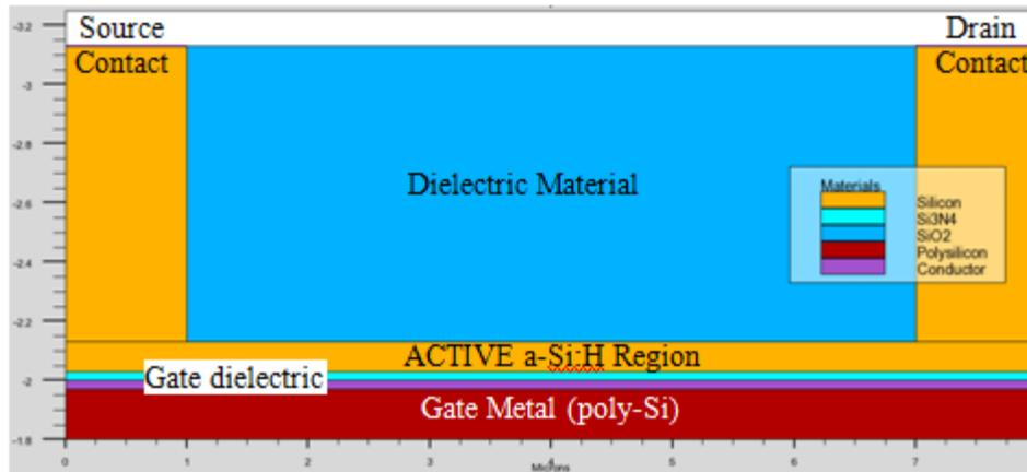
Fig.6.1 Simplified structure for simulation in Silvaco
