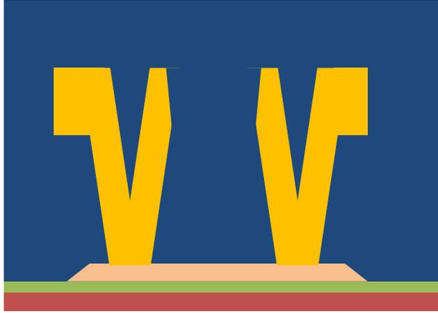
Fig. 4.10 Cross-sectional view after deposition of dielectric over terminals
