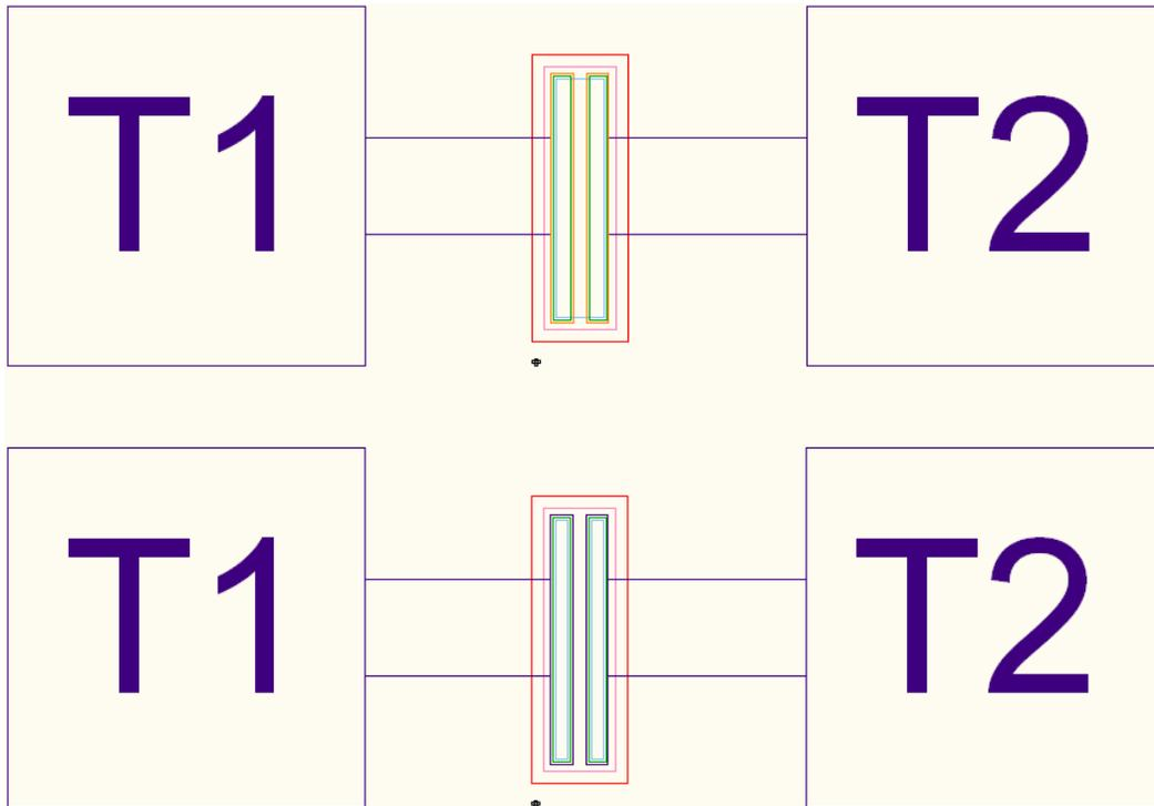
Fig. 12.7 Clean view of the resistor (a) Less resistive bypassing ACTIVE region (b) More resistive where ACTIVE region is in series connection
