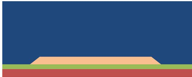
Fig. 4.6 Cross-sectional view after depositing dielectric over active region
