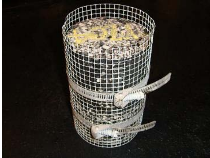
FIGURE 5. ARFC Sample Confined in Mesh Cage
