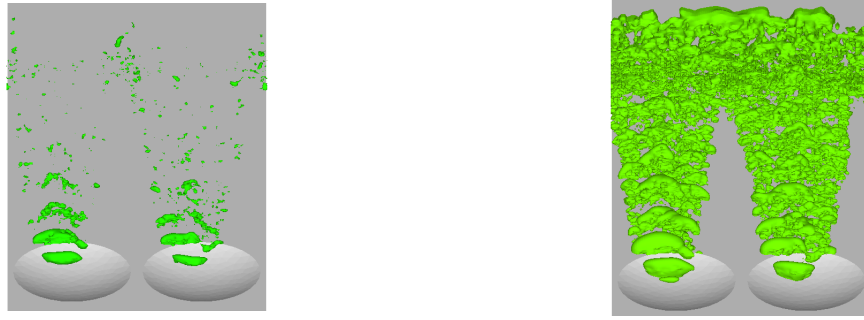
Figure 3.29. Isosurfaces of pressure for Re_\delta = 4k at t = 188 . Left: p = -0.1 ; right: p = -0.08 .
