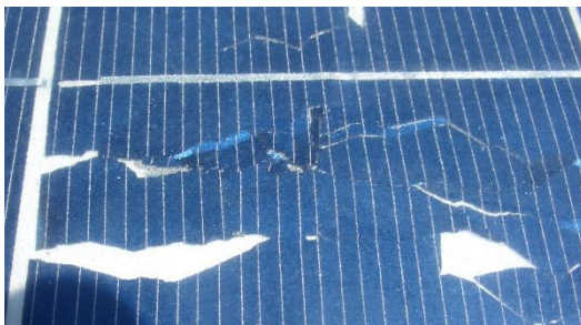
Figure 5. Shattered c-Si cell
