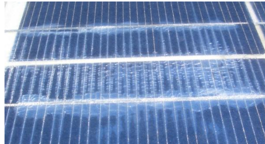
Figure 4. Delamination of encapsulant
