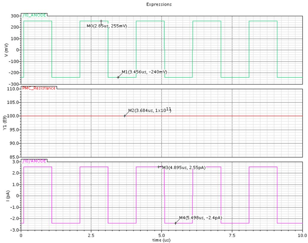
Figure 30. Waveform showing programming voltage (top) at 255mV and the current through the PMC cell limited to 400uA (middle). The cell resistance (bottom) showed NO switching to the Low resistance (ON) state as the programming voltage is below the PMC model threshold of 260mV
