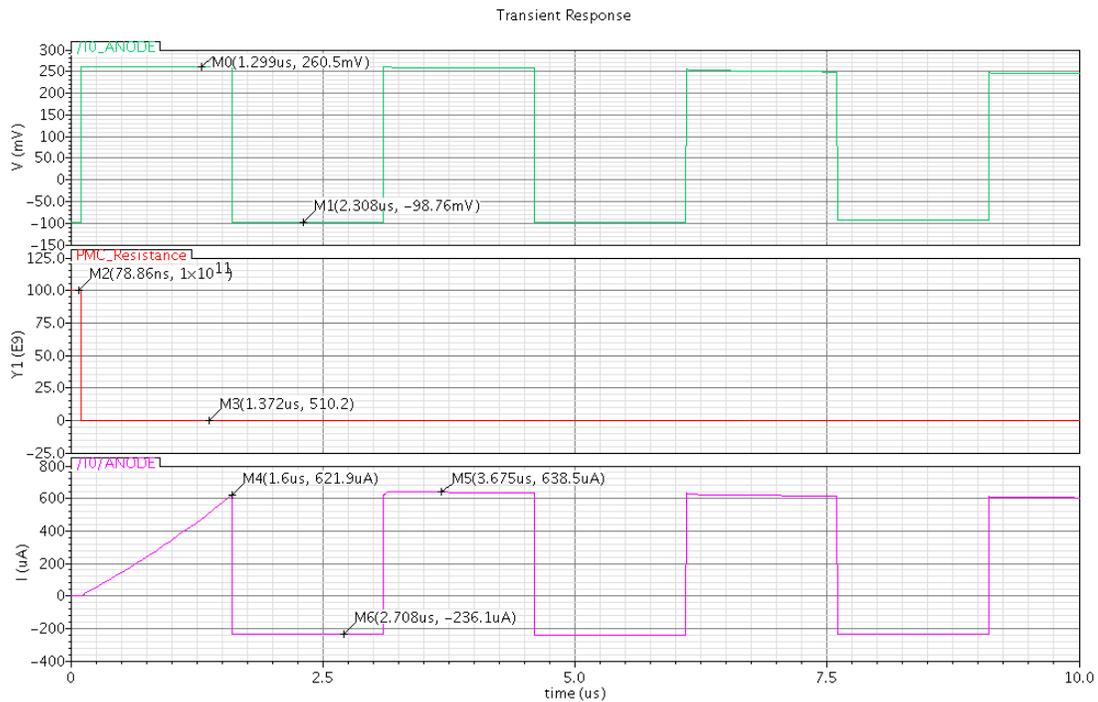
Figure 36. Waveform showing erase voltage (top) at (-99mV) and the current through the PMC cell limited to 650uA (middle). The cell resistance (bottom) showed NO switching to the high resistance (OFF) state as the erase voltage is above the PMC model threshold of -100mV
