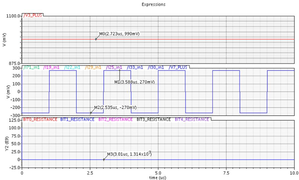
Figure 44. Showing word line voltage (top) set to 1.4v, program/erase pulse for all 8 bit lines combined (middle), and the PMC change in PMC resistance for all 8 bits (bottom). Bit line resistance remains unchanged when word line resistance is below the 1v threshold for the switches
