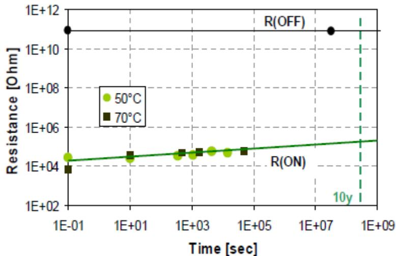
Figure 10. CBRAM data retention measured at elevated temperatures (via diameter 850nm) [14]
