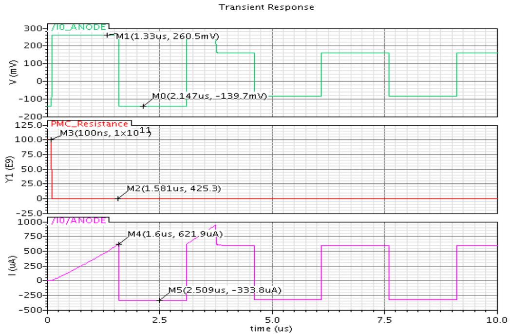
Figure 34. waveform showing waveform showing erase voltage (top) at (-140mV) and the current through the PMC cell limited to 650uA (middle).The cell resistance (bottom) showed NO switching to the high resistance (OFF) state as the erase voltage is above the PMC model threshold of -150mV
