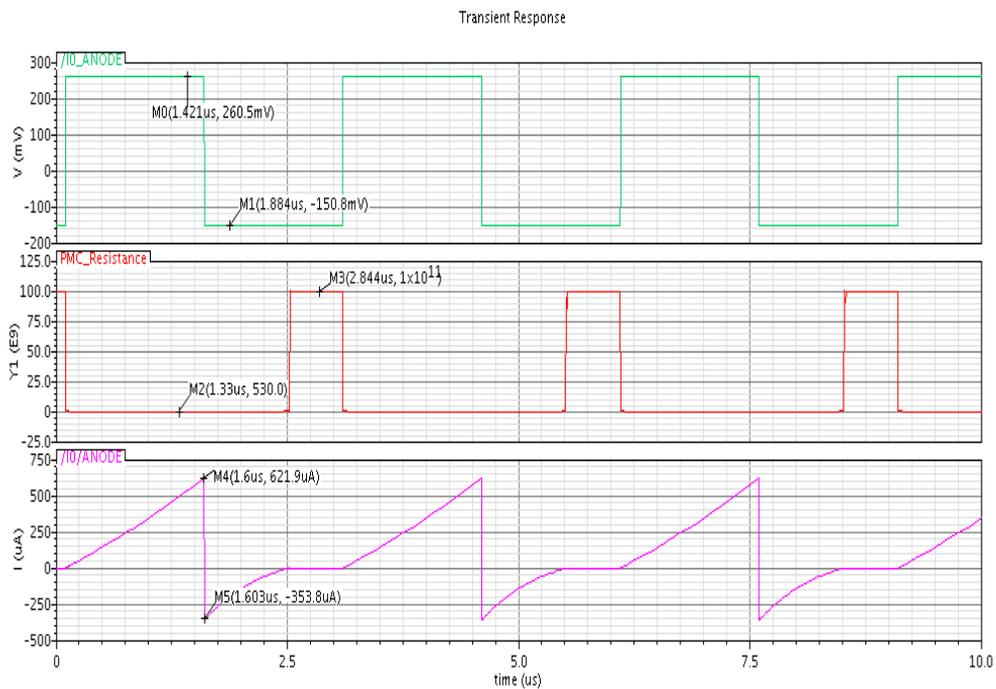
Figure 37. Waveform showing waveform showing the PMC off resistance with the model to reflecting a 10E11 OFF resistance
