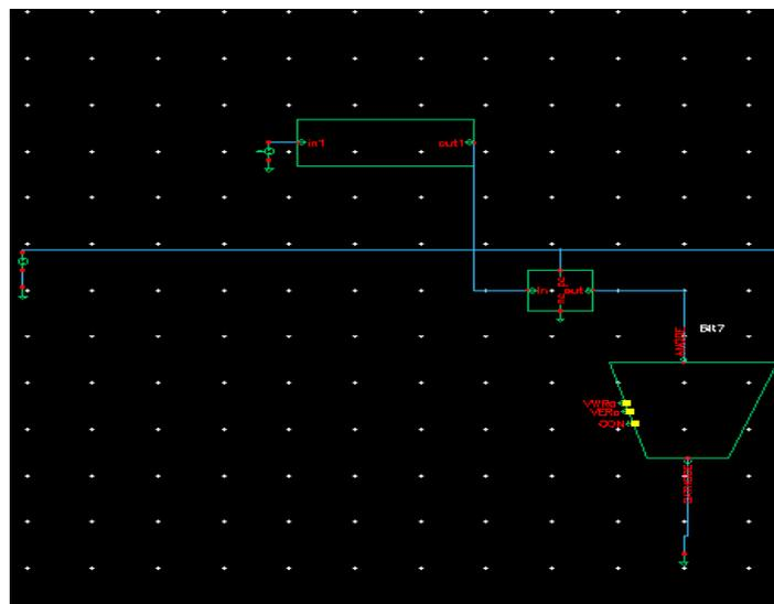
Figure 41. Showing a single PMC cell in the array connected to voltage source through a current limiter and an ideal switch model
