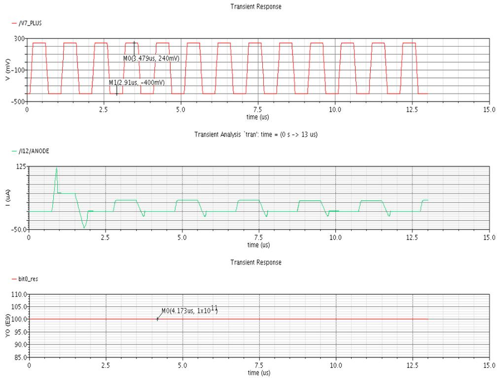
Figure 25. Waveform showing programming voltage (top) 240mV and the current through the PMC cell limited to 50uA (middle). The cell resistance (bottom) did not switch to the low resistance (ON) state as the minimum voltage of 250mV was not provided.
