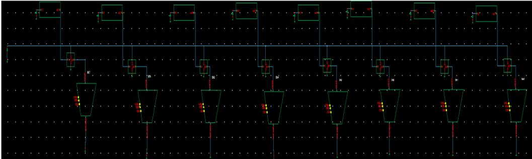
Figure 40. Showing an 8bit x1 PMC memory array
