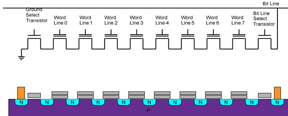
Figure 3. Flash architecture. Layout For an 8-bit NOR flash (TOP), layout For an 8-bit NAND flash (bottom) [16]
