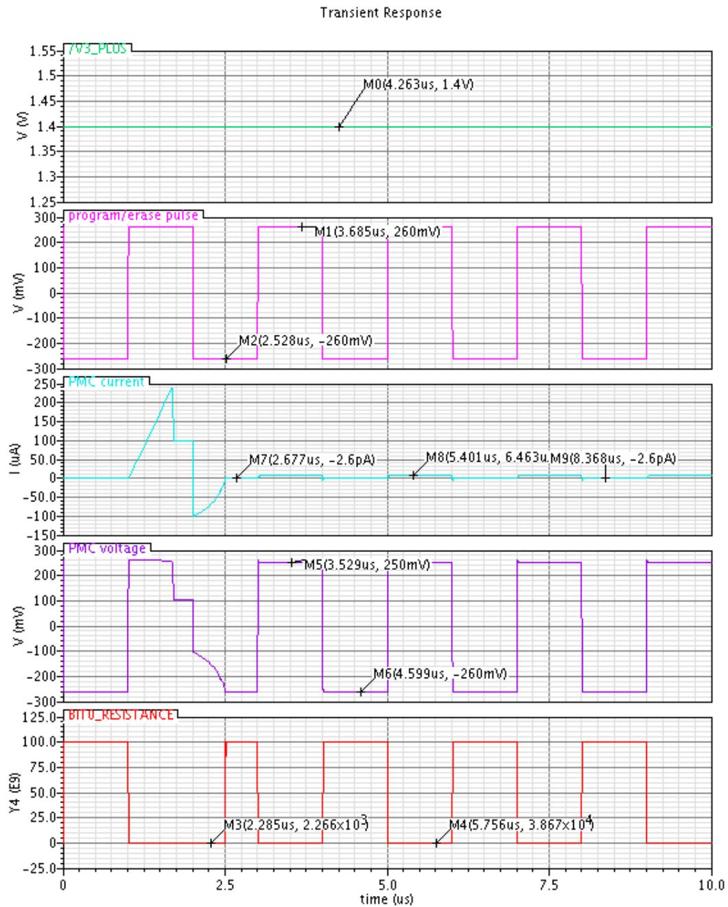
Figure 48. Showing word line voltage (top) set to 1.4v, program/erase pulse for bit0 (middle), and the PMC change in PMC resistance for bit0 (bottom). PMC input current limited to 100ua. Resulting RON is in the 38kohm range
