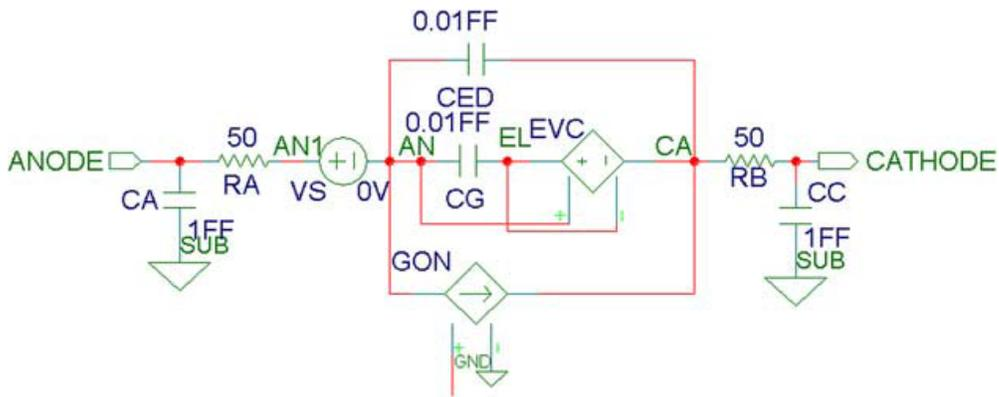
Figure 15. PMC parasitics equivalent circuit [8]
