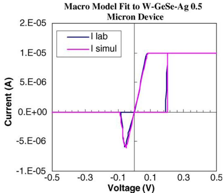
Figure 19. Results of curve fitting simulation data with experimental IV data from 4155. The device diameter was 0.5  $\mu\text{m}$ . The current limit was 10  $\mu\text{A}$ , ref [8].
