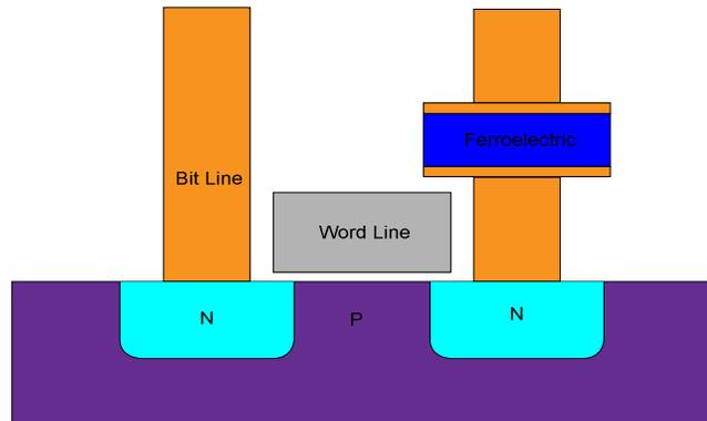
Figure 4: FERAM cell structure: the FeRAM cell structure resembles that of a 1T1C DRAM with a ferroelectric layer instead of a capacitor [16]
