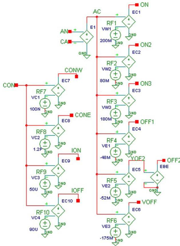
Figure 16. Comparators and thresholds for PMC switching dynamics [8]
