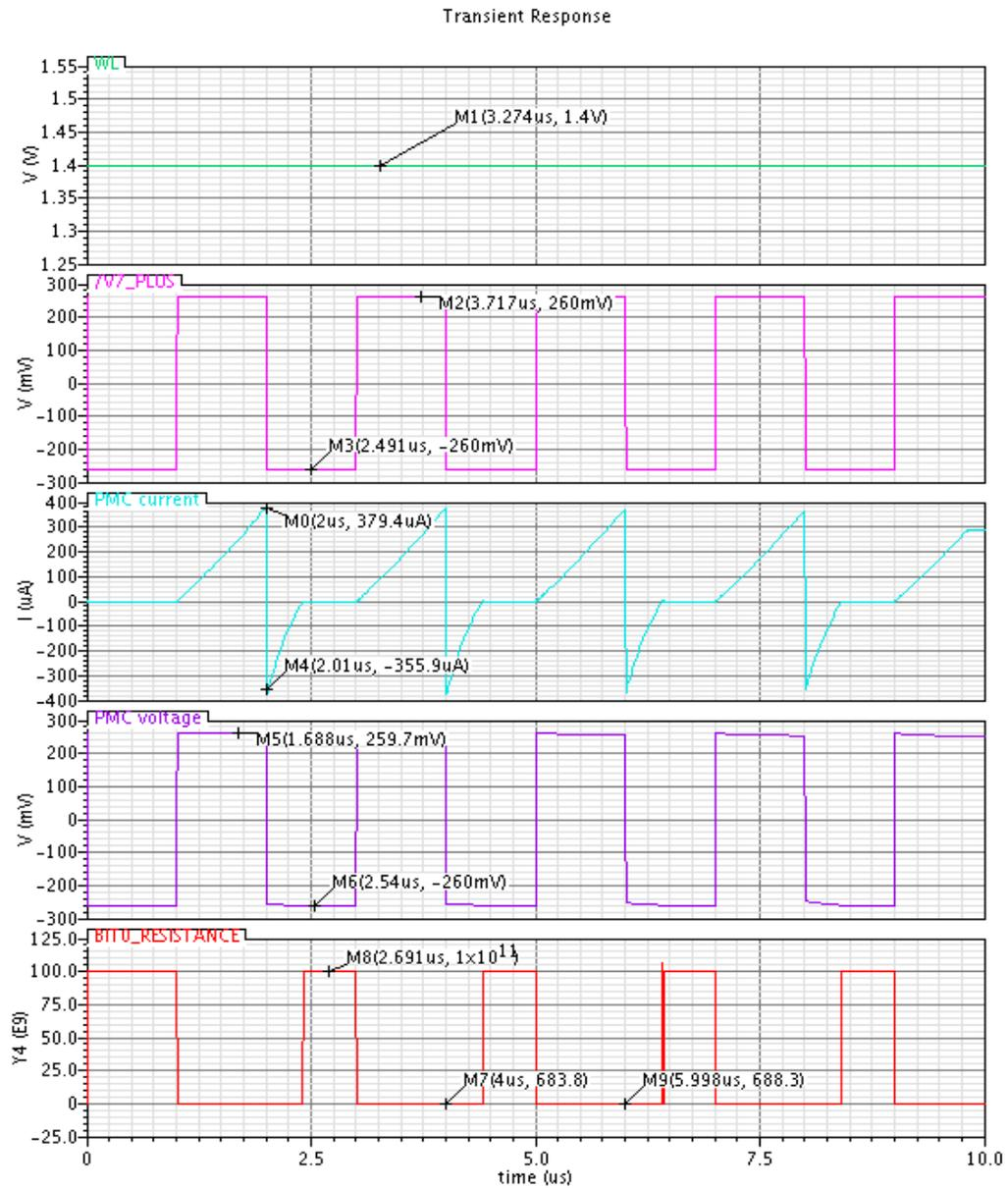
Figure 49. Showing word line voltage (top) set to 1.4v, program/erase pulse for bit0 (middle), and the PMC change in PMC resistance for bit0 (bottom). PMC input current limited to 400ua. Resulting RON is approximately 700 ohms
