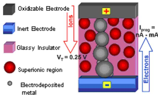
Figure 8. PMC program operation; Ion are reduced on the inert electrode forming a nano-wire (bridge) reducing the resistance of the PMC [17]
