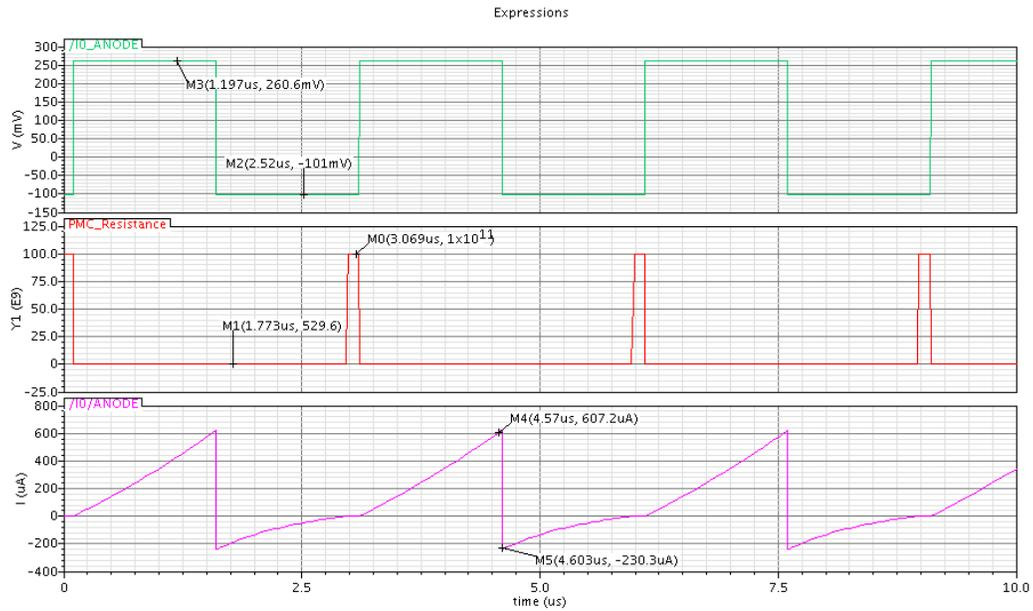
Figure 35. Waveform showing waveform showing erase voltage (top) at (-101mV) and the current through the PMC cell limited to 650uA (middle).
