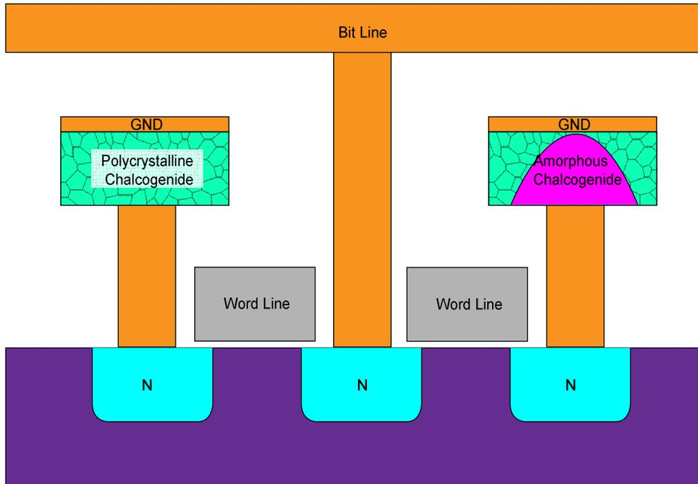
Figure 7: A cross section of two PRAM memory CELLS (One cell is in low resistance crystalline state, the other in high resistance amorphous state) [16]
