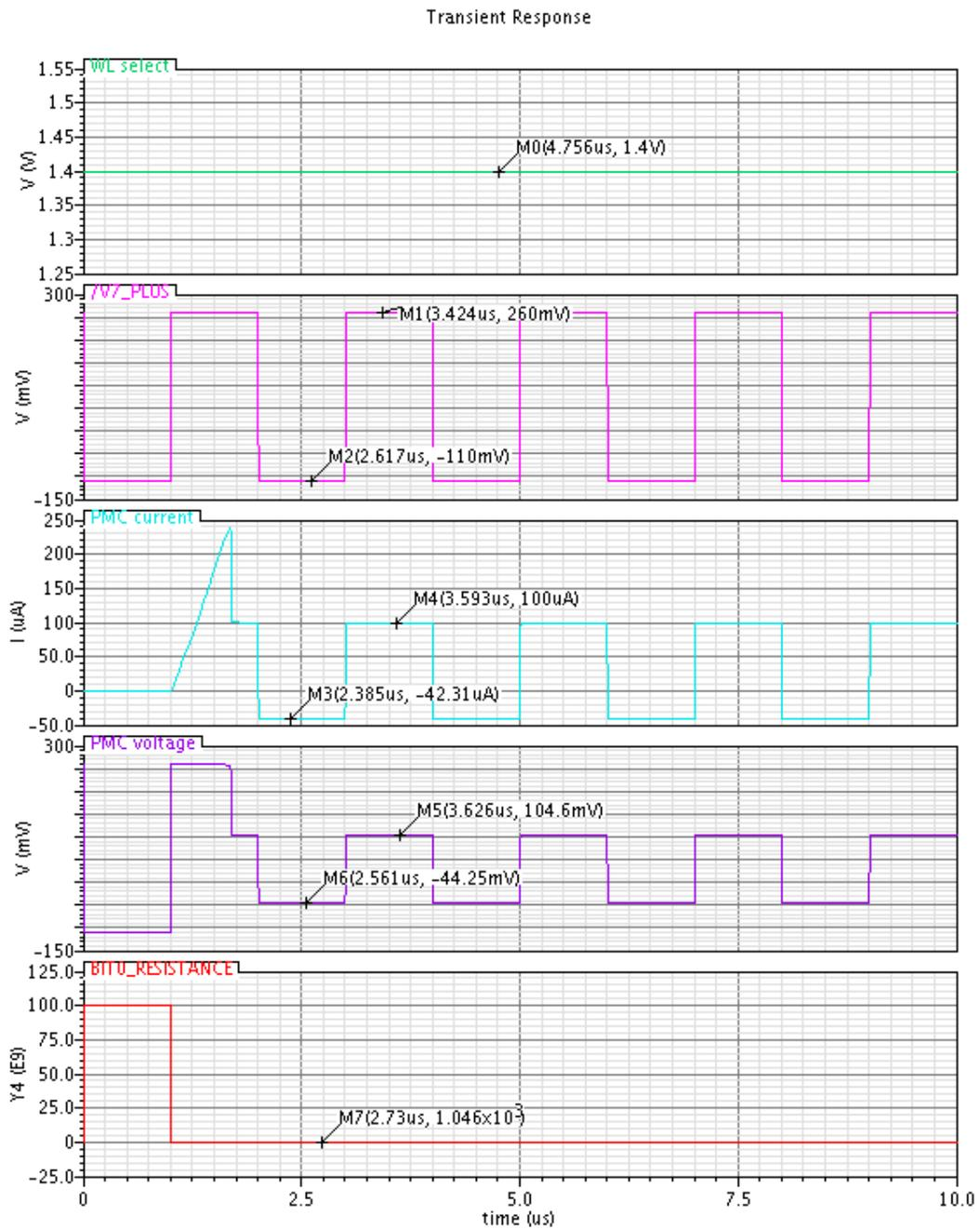
Figure 46. Showing word line voltage (top) set to 1.4v, program/erase pulse for bit0 (middle), and the PMC change in PMC resistance for bit0 (bottom). PMC input current limited to 100ua.current limit setting resulting in insufficient voltage on the PMC anode
