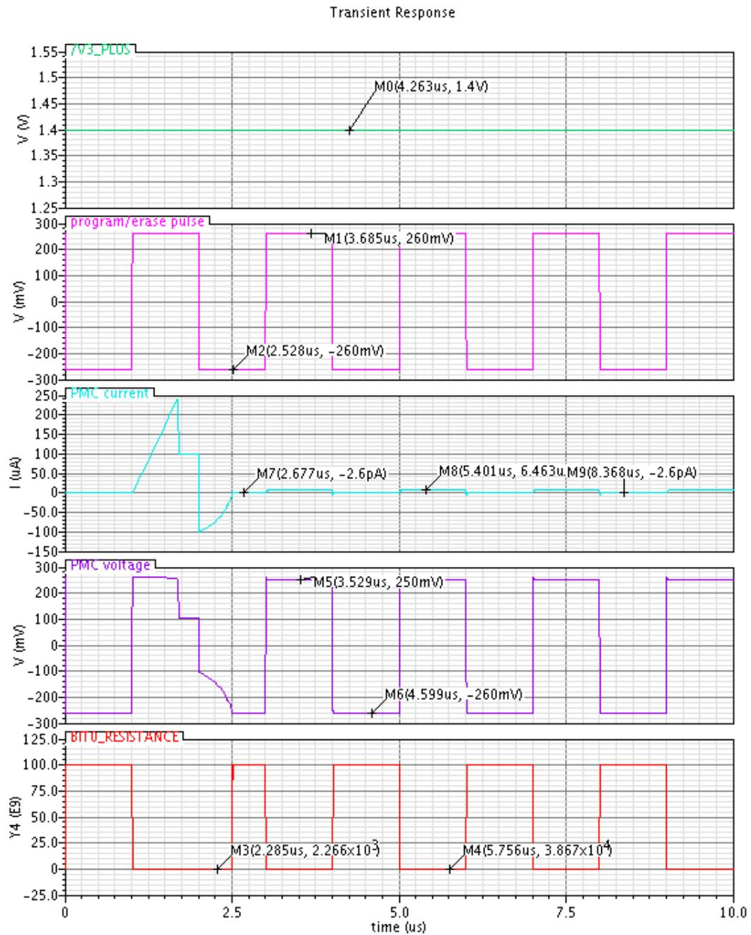
Figure 47. Showing word line voltage (top) set to 1.4v, program/erase pulse for bit0 (middle), and the PMC change in PMC resistance for bit0
