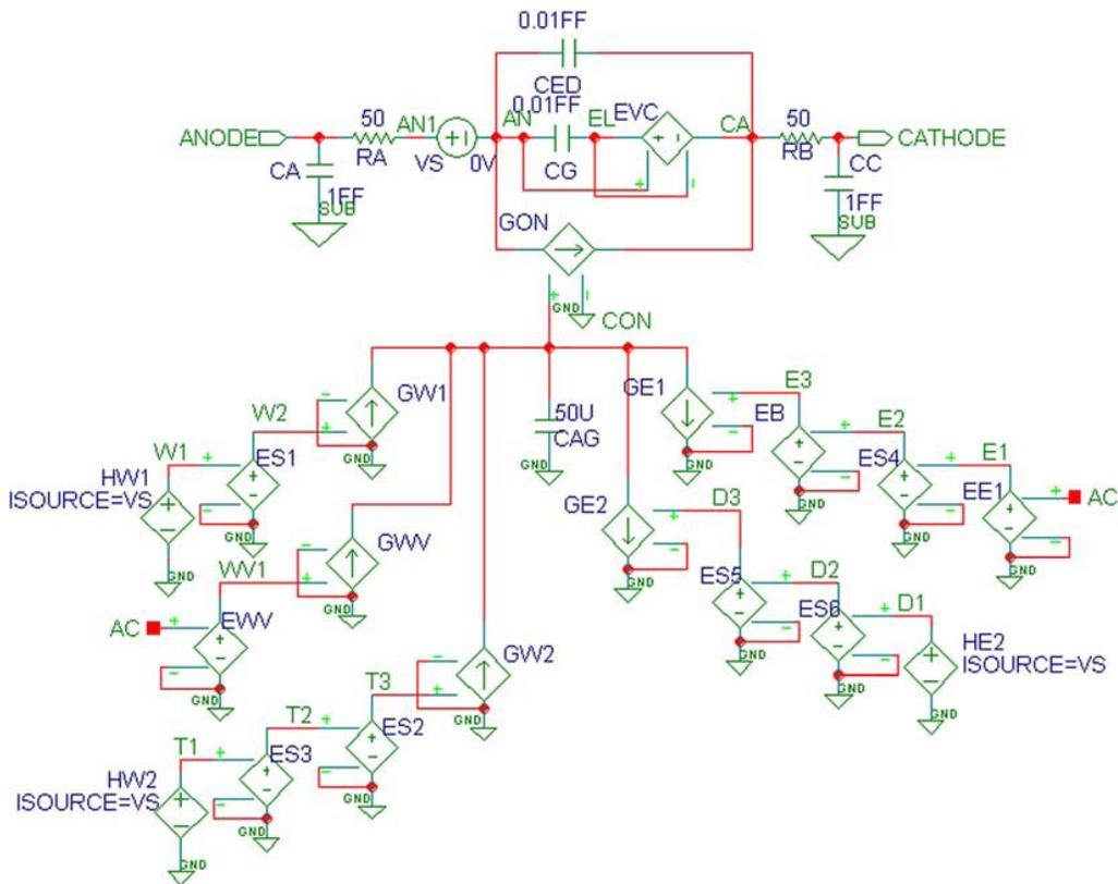
Figure 14. PMC SPICE MODEL representing the PMC single bit cell [8]
