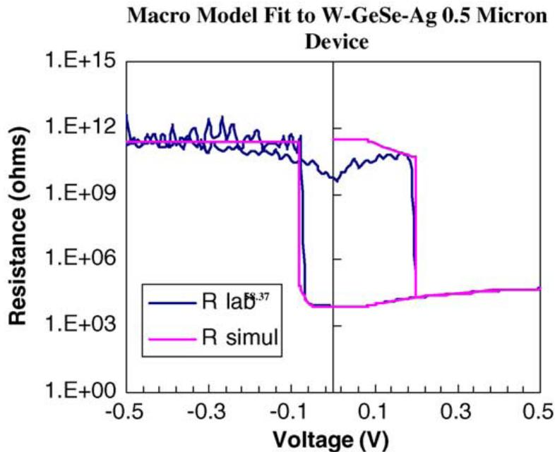
Figure 20. Results of curve fitting simulation data with experimental RV data. The device diameter was 0.5  $\mu\text{m}$ . The current limit was 10  $\mu\text{A}$ , ref [8].
