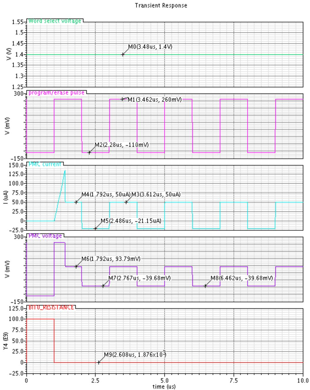
Figure 45. Showing word line voltage (top) set to 1.4v, program/erase pulse for bit0 (middle), and the PMC change in PMC resistance for bit0 (bottom). PMC input current limited to 50ua. Current limit setting resulting in insufficient voltage on the PMC anode
