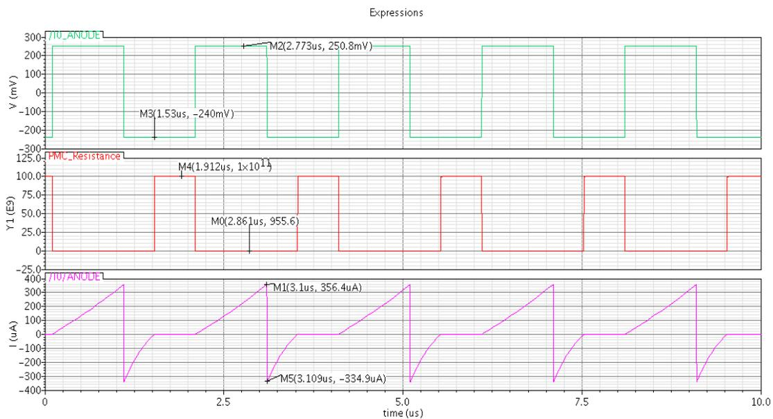
Figure 27. waveform showing programming voltage (top) at 251mV and the current through the PMC cell limited to 400uA (middle). The cell resistance (bottom) showed proper switching to the Low
