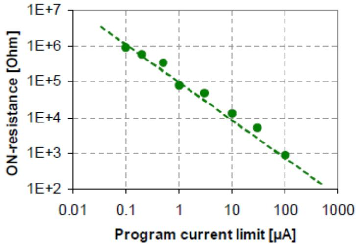
Figure 12. Dependence of the ON-state resistance on the programming current for cbram devices (via diameter 380nm) at room temperature [14]
