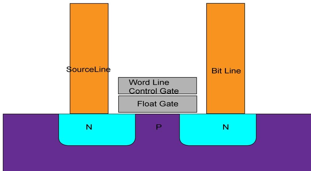
Figure 1. Flash cell structure showing a single transistor structure. This figure shows the CMOS transistor with a floating gate flash cell structure [16]
