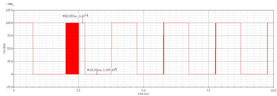
Figure 24. Waveform showing PMC cell resistance switching between OFF (high resistance state) and ON (low resistance state)
