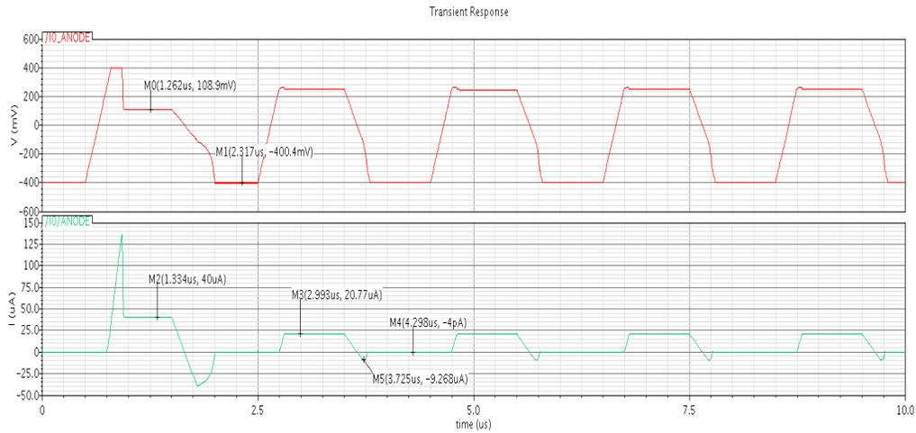
Figure 23. Waveform showing input voltage (top) and current (bottom) to the PMC cell
