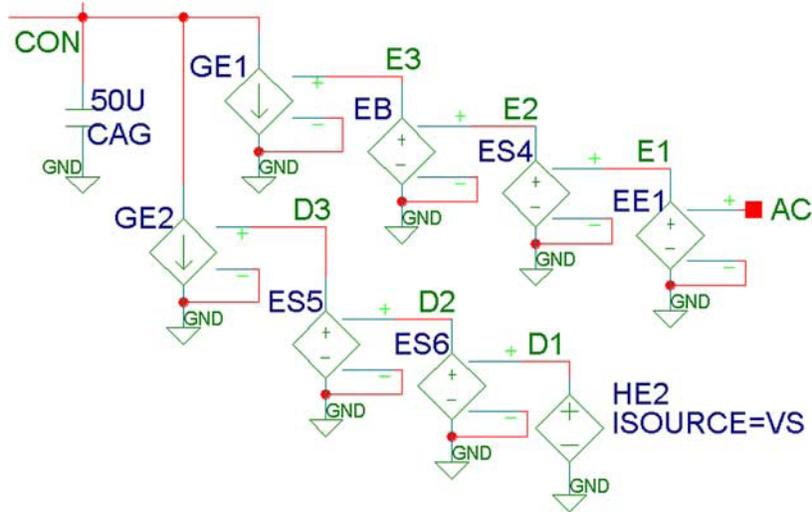
Figure 18. Dynamic erase section of SMM for PMC. The sections include the voltage and current controlled erases from top to bottom, ref [8].
