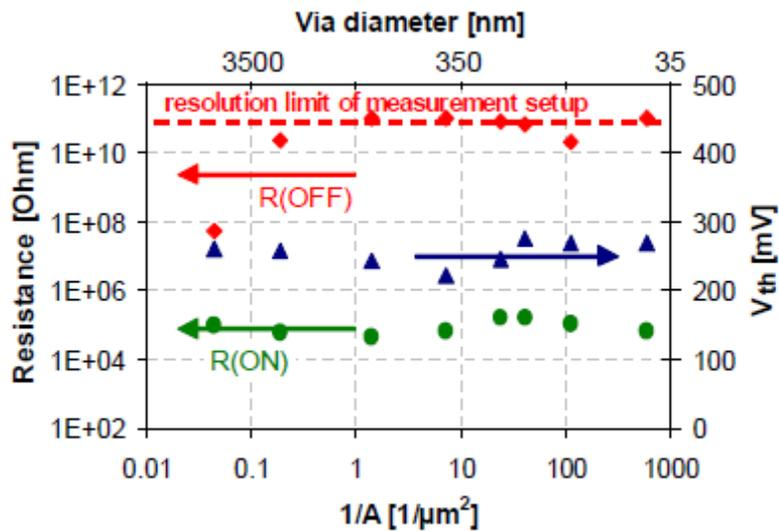
Figure 9. Scalability of CBRAM switching parameters from  $5\mu m$  to 40nm at room temperature, with the contact area  $A$  of the tungsten plug [14]
