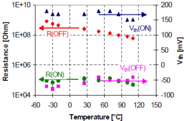
Figure 11. CBRAM switching parameter at different operating temperatures (viadiameter 380nm) [14]
