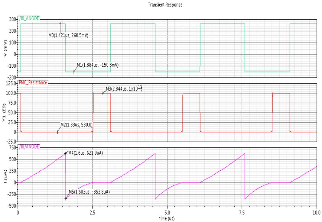
Figure 33. Waveform showing waveform showing erase voltage (top) at (-151mV) and the current through the PMC cell limited to 650uA (middle). The cell resistance (bottom) showed proper switching to the high resistance (OFF) state as the programming voltage is below the PMC model threshold of -150mV
