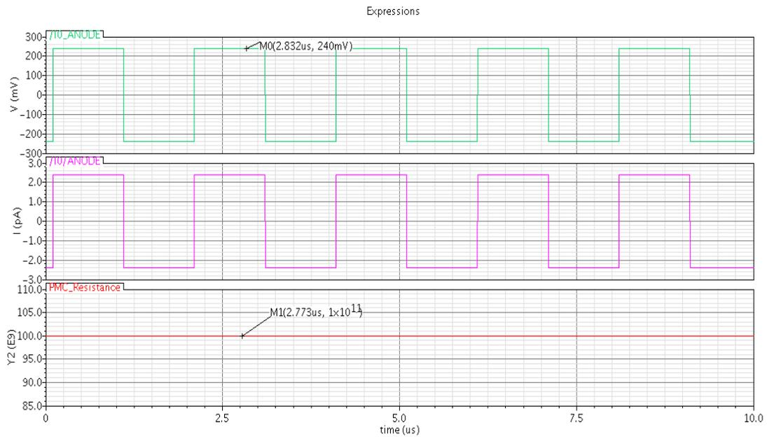
Figure 28. Waveform showing programming voltage (top) at 240mV and the current through the PMC cell limited to 400uA (middle). The cell resistance (bottom) showed NO switching to the Low resistance (ON) state as the programming voltage is below the PMC model threshold of 250mV
