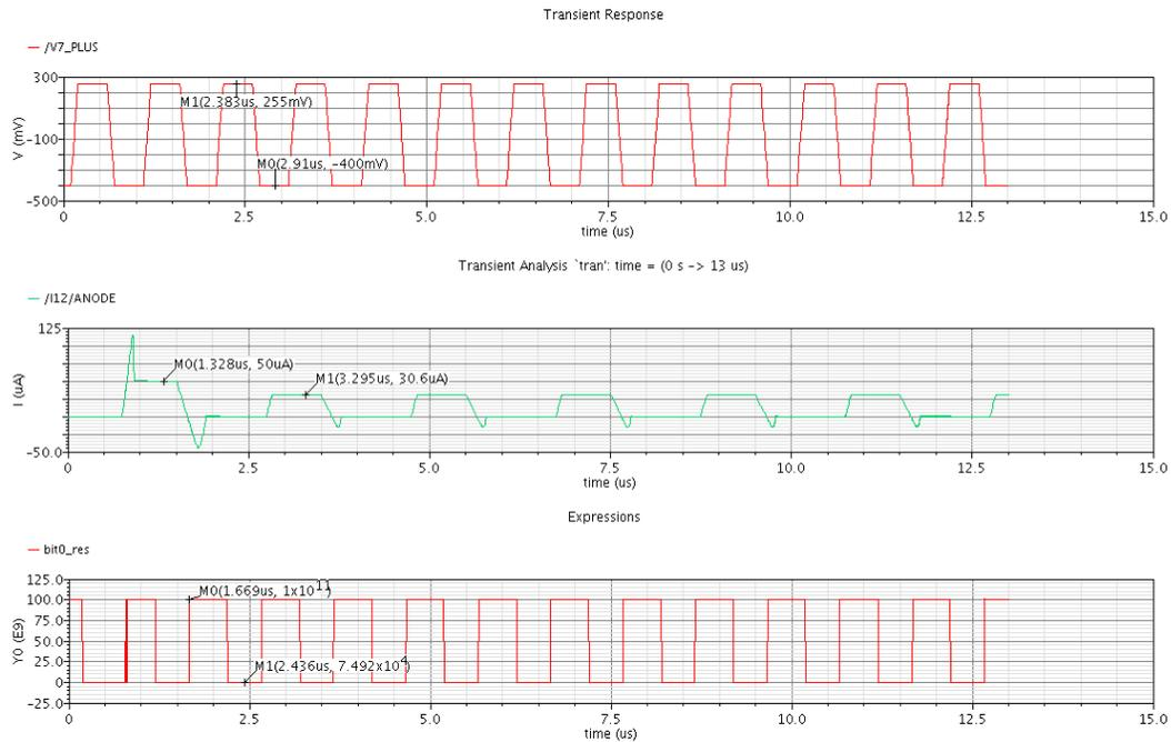
Figure 26. Waveform showing programming voltage (top) 255mV and the current through the PMC cell limited to 50uA (middle). The cell resistance (bottom) showed proper switching to the low resistance (ON) state as the programming voltage was above the minimum voltage required to initiate the electro-deposition process
