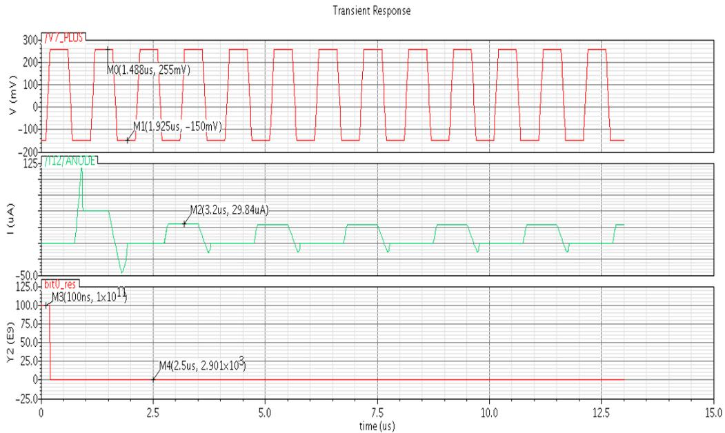
Figure 32. Waveform showing erase voltage (top) at -150mV and the current through the PMC cell limited to 50uA (middle). The cell resistance (bottom) showed proper switching to the High resistance (OFF) state as the erase voltage was set below the minimum voltage required to dissolve the conductive bridge
