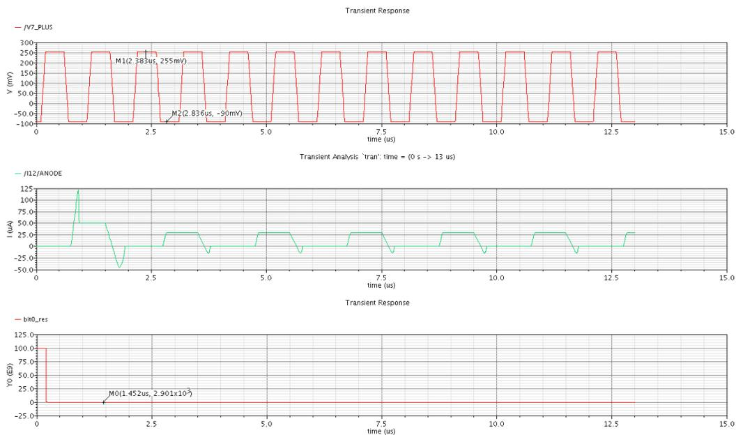
Figure 31. Waveform showing erase voltage (top) set to -90mV and the current through the PMC cell limited to 50uA (middle). The cell resistance (bottom) did not switch to the High resistance (OFF) state as the minimum voltage of -90mV was not provided.
