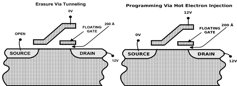
Figure 2. NOR Flash erase and program. Left diagram shows the erase process through tunneling. Right diagram shows voltages on drain and gate to trap charge via Hot Electron Injection [16]
