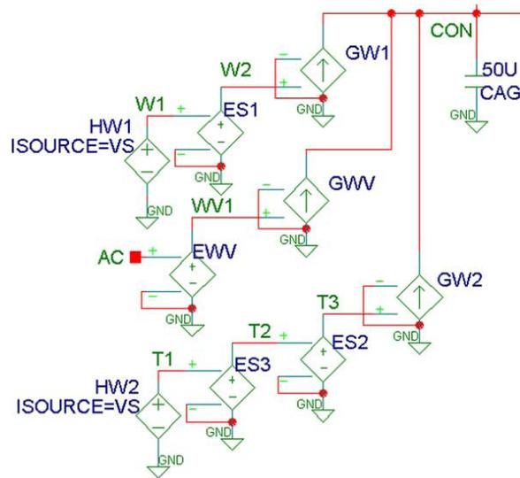
Figure 17. Dynamic write section of SMM for PMC. The sections include, FROM top to bottom, the first threshold current controlled, voltage controlled, and secondary threshold current controlled write operations [8].
