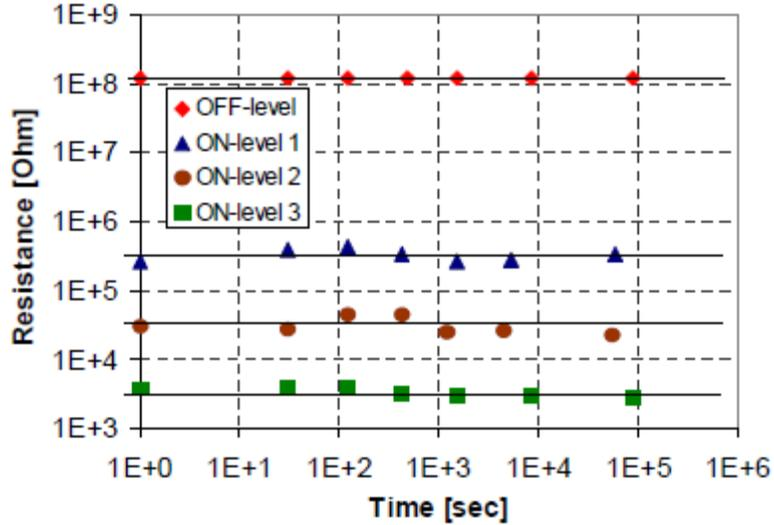
Figure 13. CBRAM multi-level capability, programming currents for ON-levels 1: 0.5μA, 2: 2μA, and 3: 20μA, respectively (via diameter 100nm) [14]
