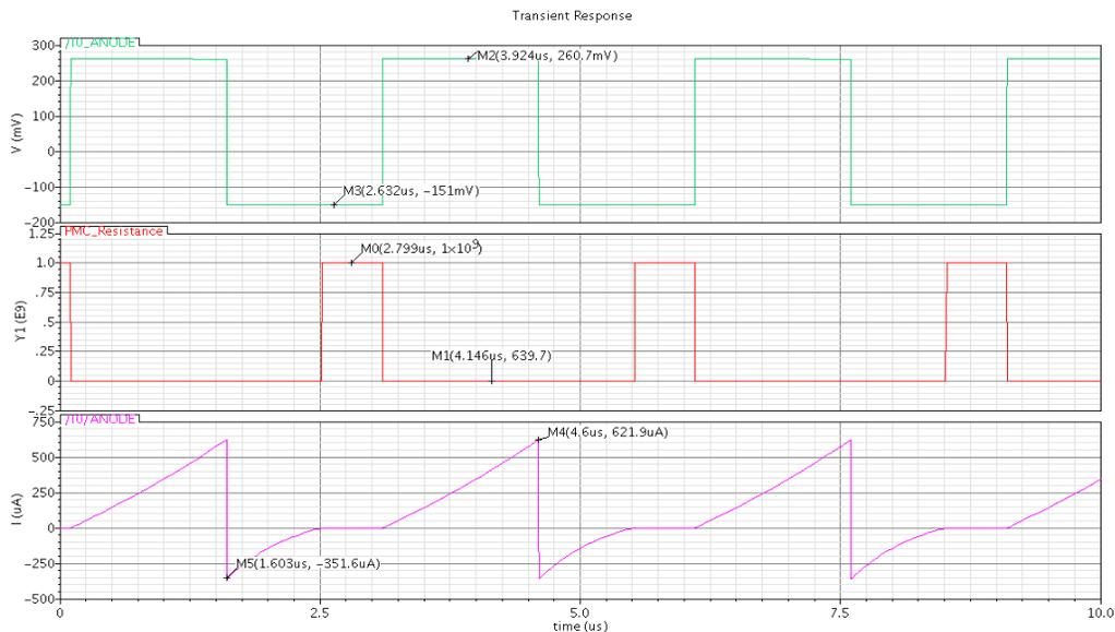
Figure 38: waveform showing waveform showing the PMC off resistance after modifying the model to reflect a 10E9 Ohm off resistance form a 10E11
