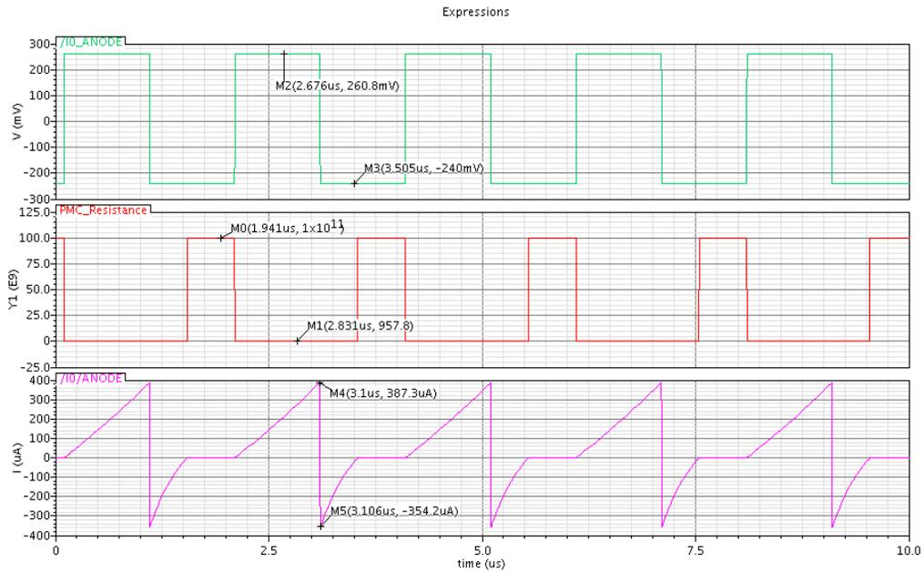
Figure 29. waveform showing programming voltage (top) at 261mV and the current through the PMC cell limited to 400uA (middle). The cell resistance (bottom) showed proper switching to the Low resistance (ON) state as the programming voltage is above the PMC model threshold of 260mV
