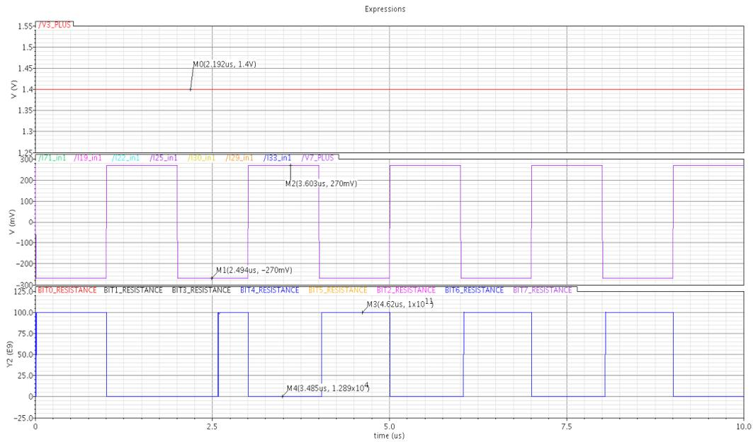
Figure 42. Showing word line voltage (top) set to 1.4v, program/erase pulse for all 8 bit lines combined (middle), and the PMC change in PMC resistance for all 8 bits (bottom) bit line resistances can be programmed when word line resistance is above the 1v threshold for the switches.
