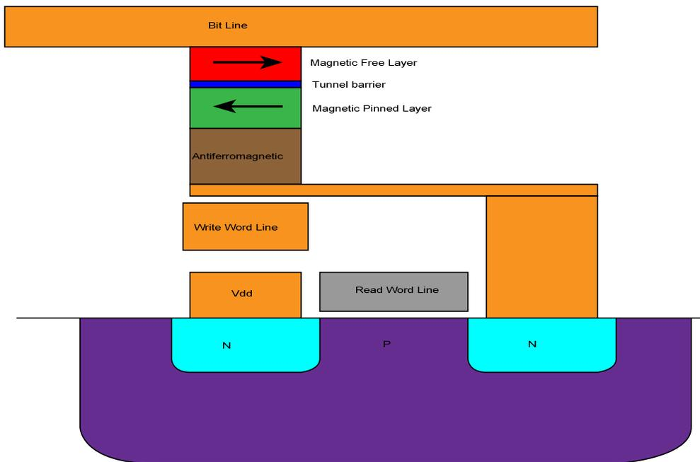
Figure 6: MRAM cell structure showing the programmable cell is placed between two write lines at right angles from each other. The anti-ferromagnet layer is used in “toggle mode” [16]
