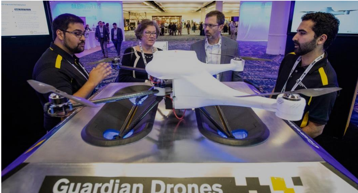
Figure 4. Seen above, Luminosity students developed and submitted an invention disclosure for a base station capable of automatically docking and charging the guardian drones through a contact-driven system (Photo by Charlie Leight/ASU Now).
