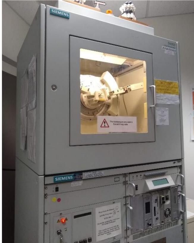
Figure 2-5: Siemens D-5000 Powder X-ray Diffractometer utilized in this study.
