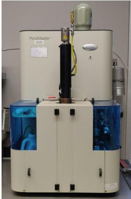
Figure 2-3: Quantachrome Instruments Pore Master mercury intrusion porosimeter utilized in this study.
