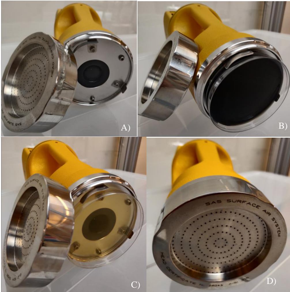
Figure 1A: Illustration of Bioscience International Microbial Air Sampler A) without Plate B) with BCYE Plate Inserted C) with TSA Plate Inserted and D) Assembled
