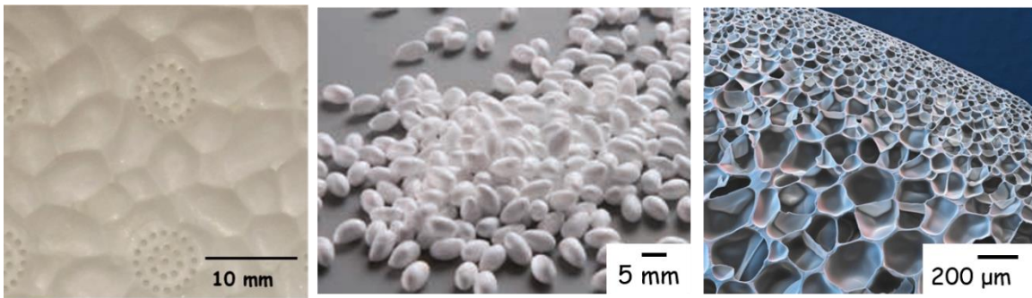
Figure 1: Photograph of the molded foam beads with hundreds of individual beads which are themselves composed of microcells (from left to right).
