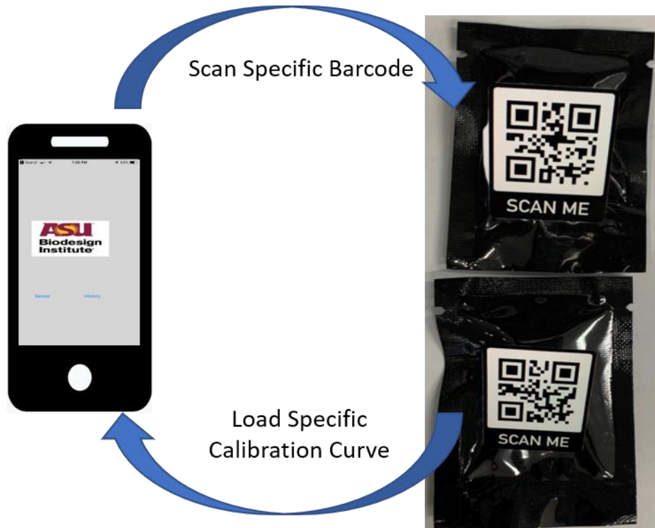
Figure 53: QR scanning of specific biomarker with smartphone device. Corresponding calibration curves and threshold values are loaded.
