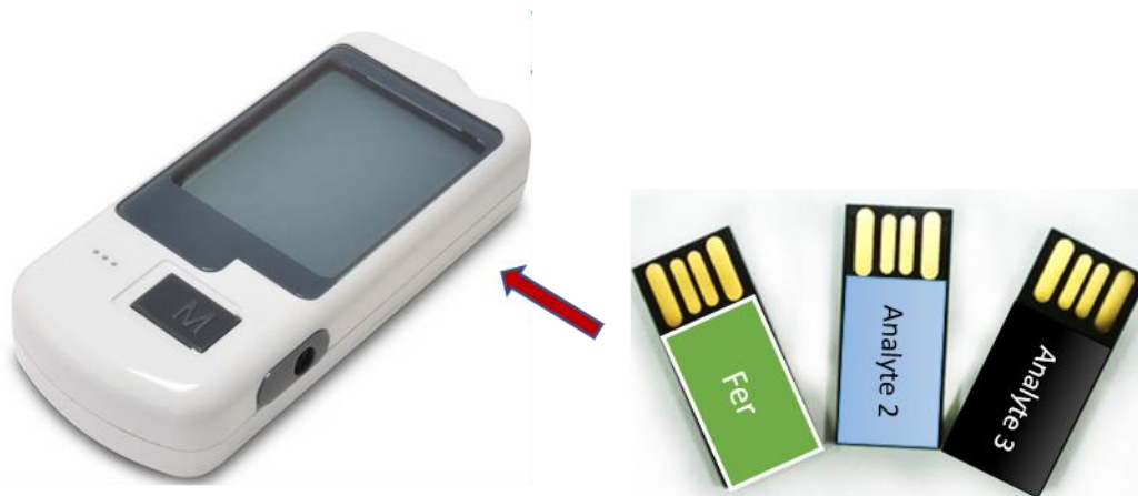
Figure 54: A chip associated with a specific biomarker is inserted into the glucometer like device and the corresponding calibration data and threshold values are loaded.
