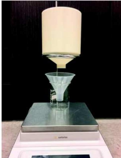
*Figure 6. Experimental set-up showing the 3D printed hopper clamped to a stand and placed above a balance with beaker.*
