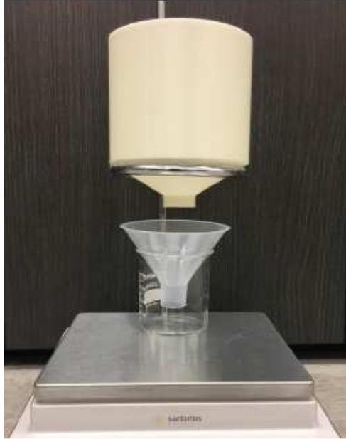
*Figure 14. Experimental setup of the hopper. Clamped 3D-printed hopper with a beaker, for collecting discharged particles, placed on an analytical balance to measure the mass of discharged particles for sampling (Chen et al., 2017).*
