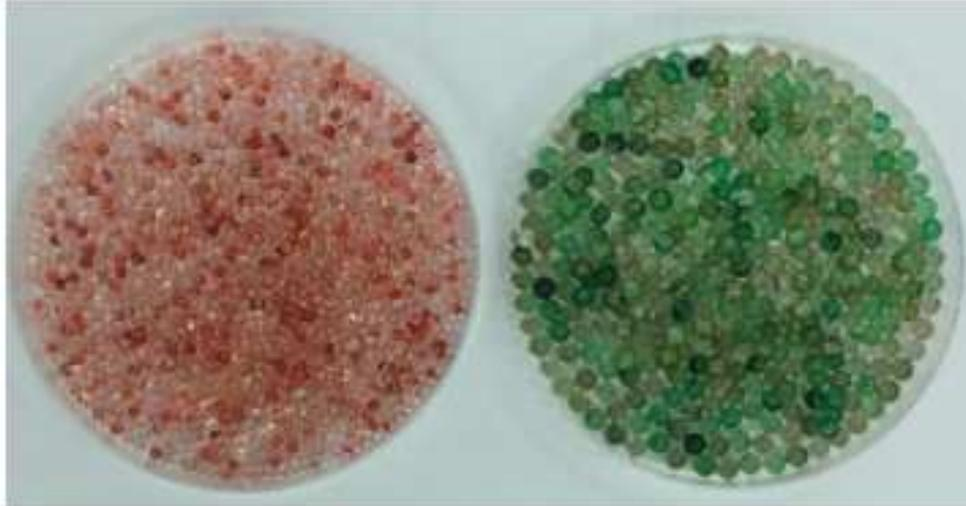
*Figure 8. Silica beads: Normal distribution of the fine particles with mean of 1.5 mm and standard deviation of 0.3 mm, colored in red; and the coarse particles with a mean of 2.9 mm and standard deviation of 0.1 mm, colored in green.*
