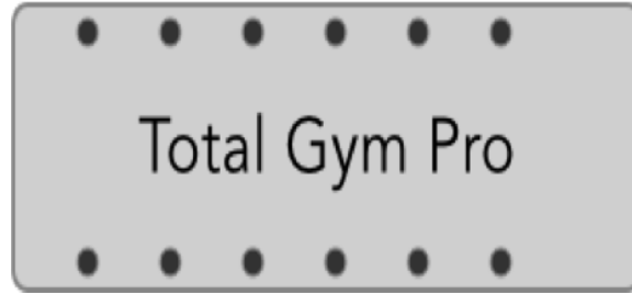
Figure 5.3: Location of the Pressure Sensor and Pancake Motor Pairs Along the Outside of the Total Gym Pro (Tadayon et al. , 2017).
