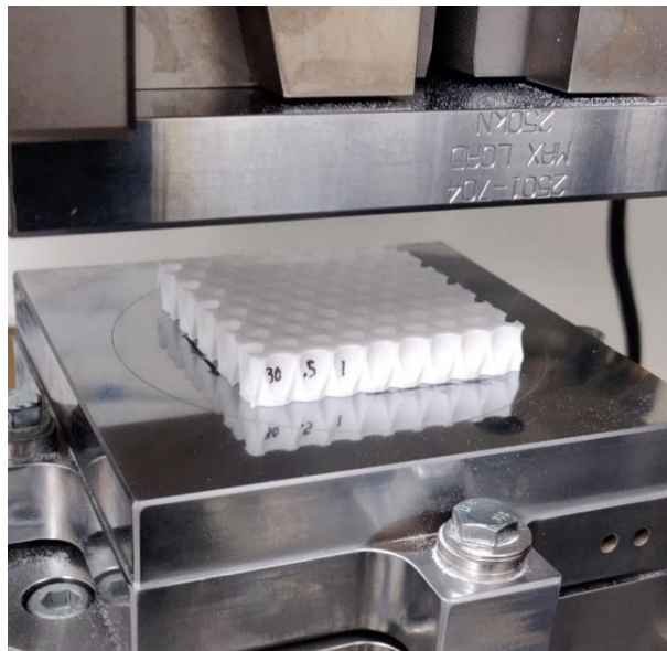
Figure 45: Compression platens with sample
