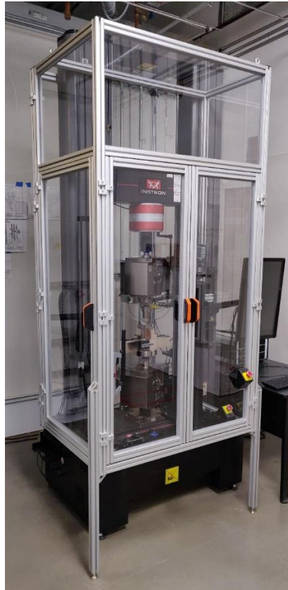
Figure 44: Instron 5985 250kN Load Frame
