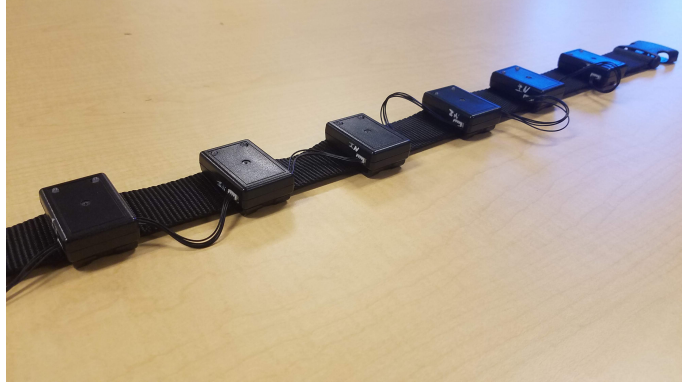
Figure 3.3: Haptic Belt developed at the CUbiC Lab at Arizona State University Rosenthal et al. (2011). The belt was designed to be modular and can be extended to fit more or fewer tactors connected in series. The location of the tactors can also be modified by simply sliding them along the belt.
