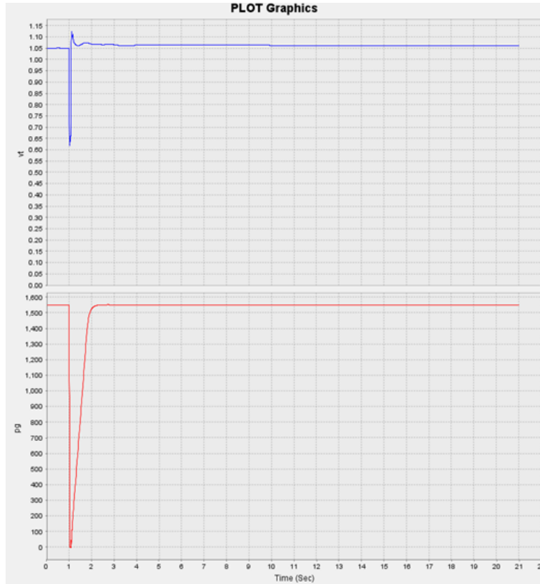
Figure 4.3: The performance of power generation the unit shown in Fig 4.2 above, notice the power generation drops to 0 when the voltage goes below 0.85
