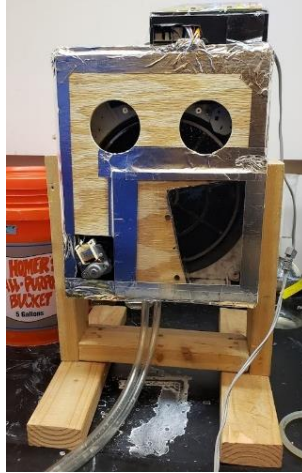
Figure 8-4 Electrical desiccant dehumidifier system with desiccant wheel containing 5w/w% carbon black enabled silica gel
