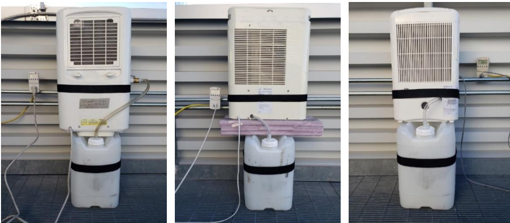
Figure 5-3 C1, D1 and D2 electric dehumidifiers placed above 5-gallon collection container (left to right)
