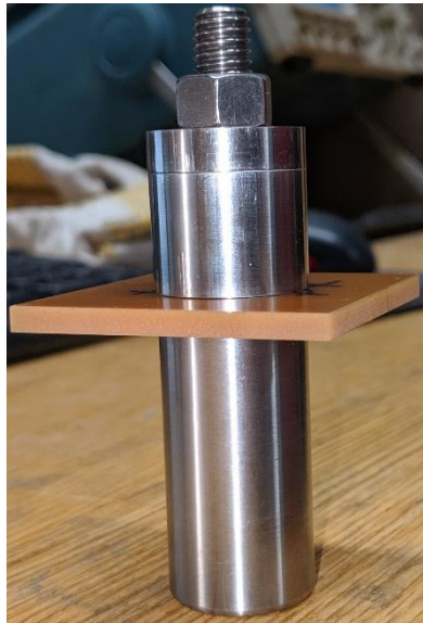
4.27 Specimen Placed on Punch Tool
