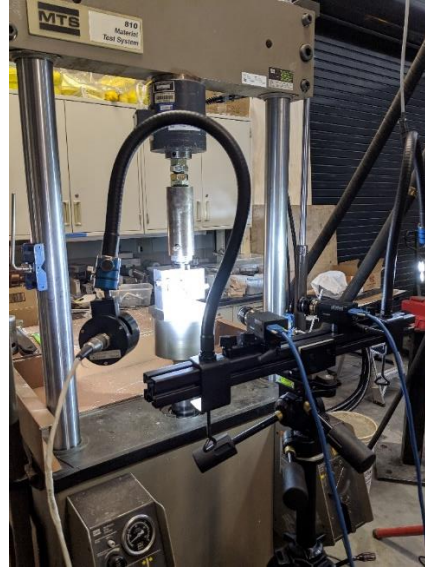
3.5 Typical DIC Camera Setup
