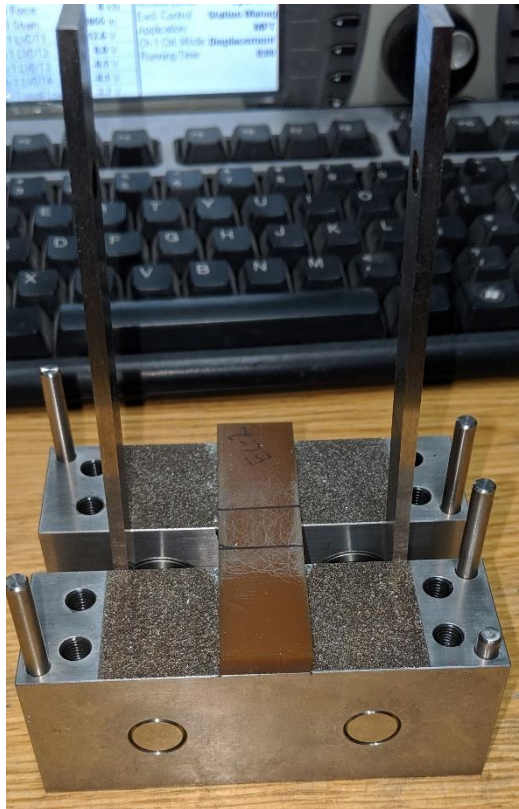
4.8 Specimen Centered on Bottom Half of Fixture with Alignment Plates
