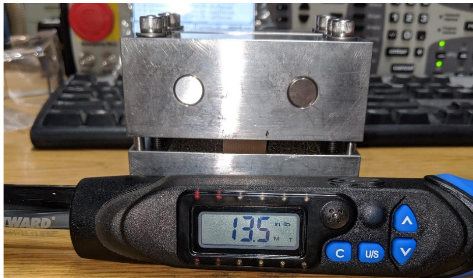
4.10 Fixture Tightened with Digital torque Wrench Used
