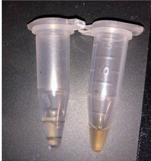
Figure 9: Eppendorf tubes holding metallic platinum reduced from ions by  $\text{NaBH}_4$  in the absence of protein (left) and platinum nanoparticles in the presence of GroEL (right)
