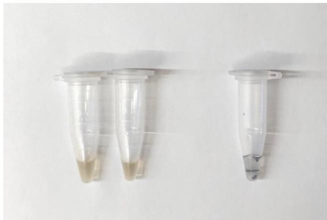
Figure 12: Low contrast photograph of platinum nanoparticles versus bulk platinum
