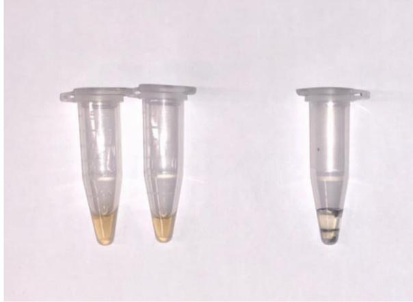
Figure 11: Eppendorf tubes showing the comparison of platinum nanoparticle formation using GroEL (two tubes on the left) versus bulk platinum formation in the absence of GroEL
