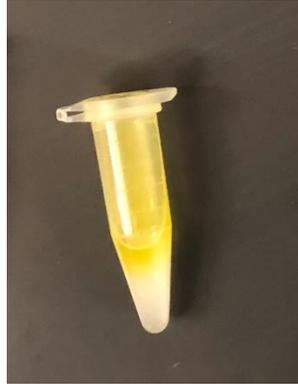
Figure 22: Eppendorf tube after incubation with ONPG showing the silica resin region displaying very little to no yellow color but the supernatant showing a bright yellow color
