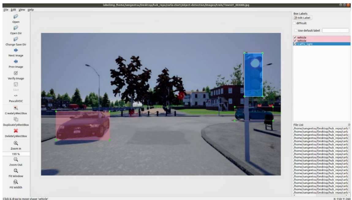
Figure 18 – Annotating a Sample Image Using Labellmg
