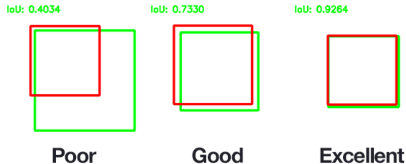
Figure 22 - An example of computing IoU for various bounding boxes
