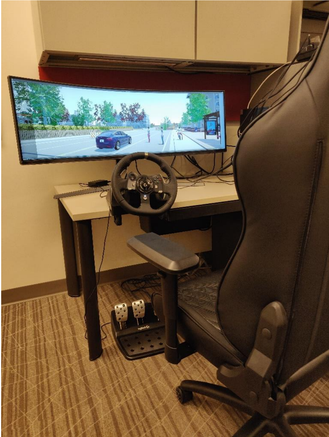
Figure 13 – Driving Simulator Setup
