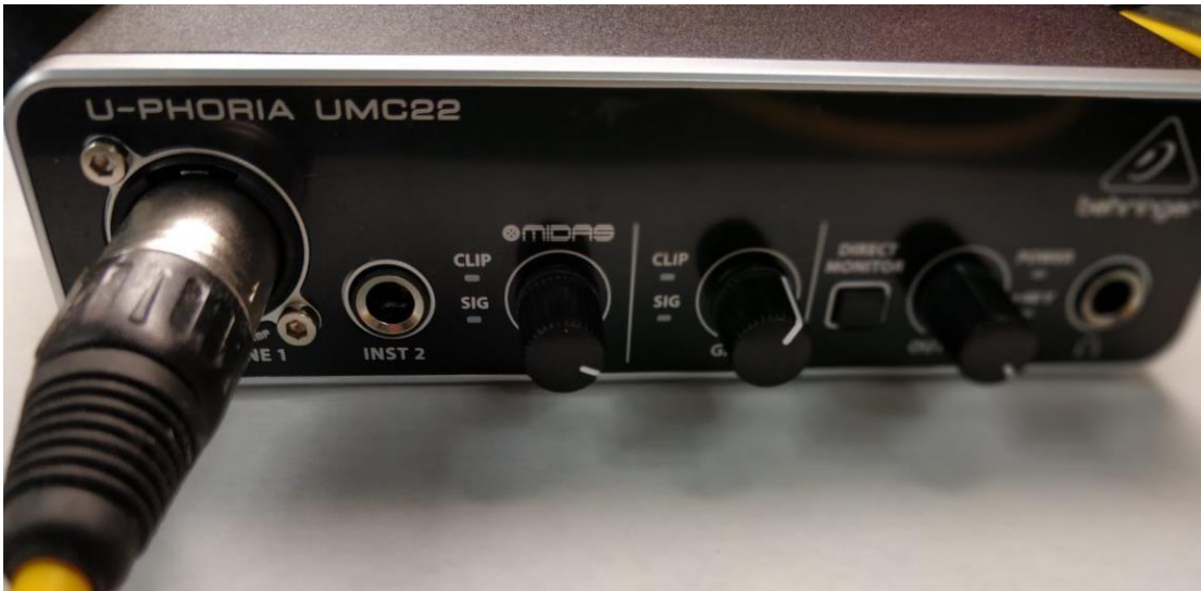
Fig 5 : Audio USB interface, behringer u-phoria umc22
