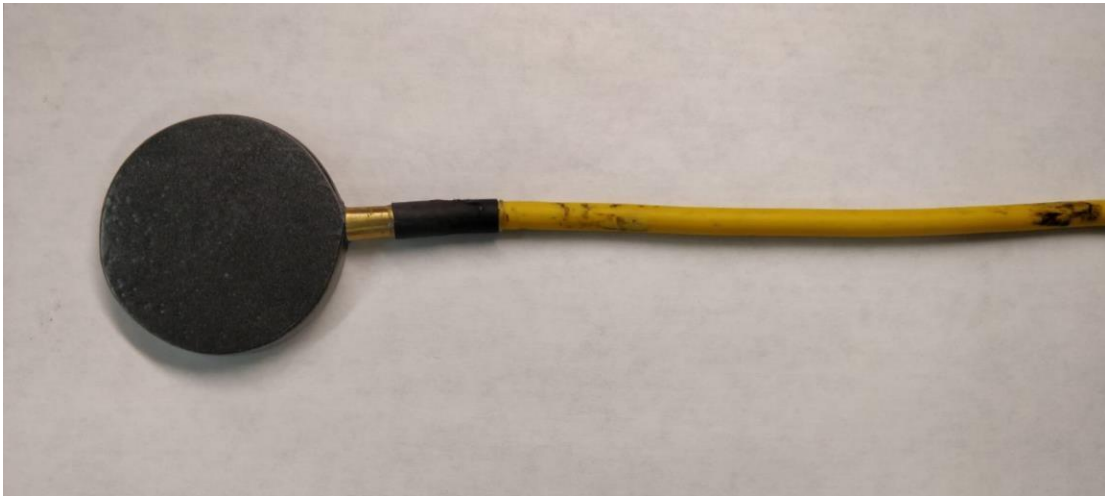
Fig 4 : Hydrophone, DolphinEar PRO Series
