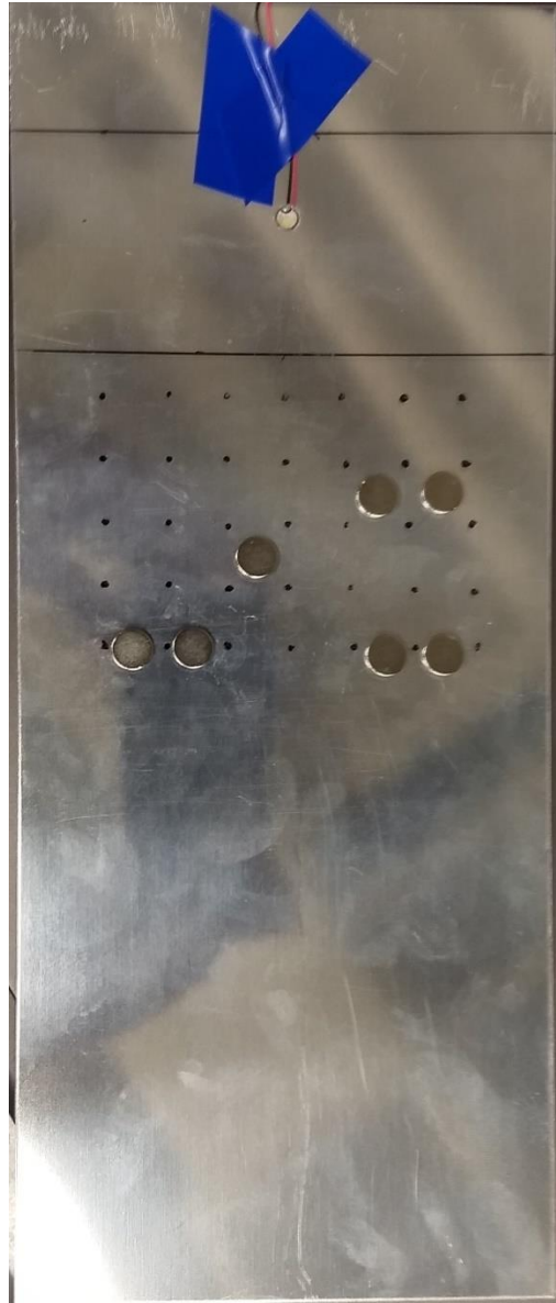
Figure 7 The position of the added masses has been indicated in this picture. The additional masses are added at the back of the sample
