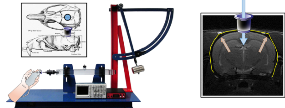
Figure 3 FPI Device. An Implanted Cranial Hub is Attached to the Injury Device Where an Adjustable Pendulum Falls and Strikes the Plunger, Generating a Fluid Pulse That Impacts the Dural Surface, Resulting in a DAI Without Cavitation or Contusion
