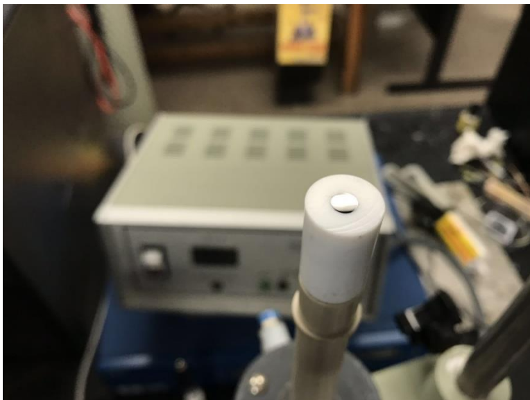
Figure 8. Polished RDE working electrode.
