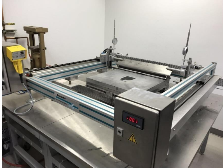
Figure 15. EC26 Coatema machine with the carbon slurry coated carbon paper.
