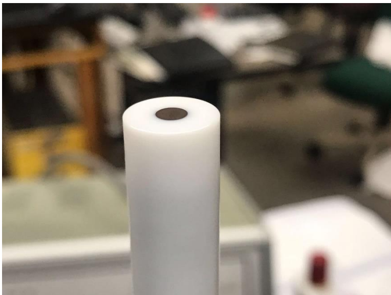
Figure 10. Thin film on RDE.
