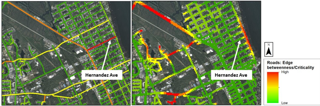
Figure 5.4. Traditional (5.4a) and modified (5.4b) criticality measurements for a portion of the study area. Note the anomalously high edge betweenness criticality for the relatively short Hernandez Avenue. This is due to missing connectivity data in the underlying road shapefile. The modified grid-based approach corrects for this error.
