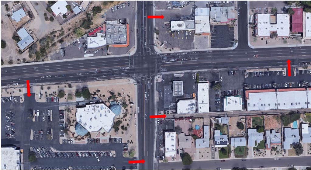
Figure 4.1. An illustration of how off-network features (such as parking lots, alleys, and driveways) provide de facto street network connectivity.
