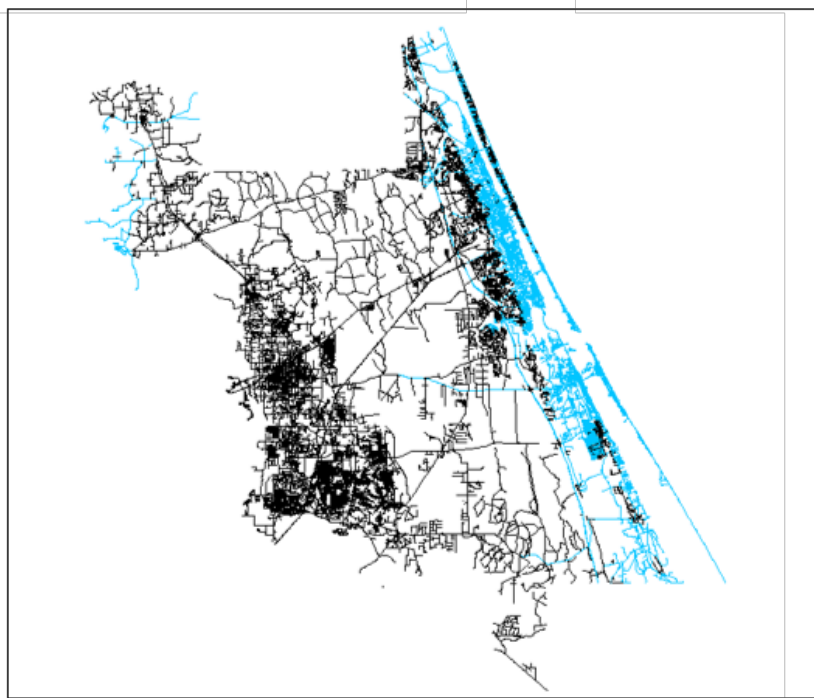
Figure 3.3. Road network degradation in Volusia County for Category II (a) and IV (b) hurricane storm surges. Light blue roads are those that are washed out. Black roads are still intact.
