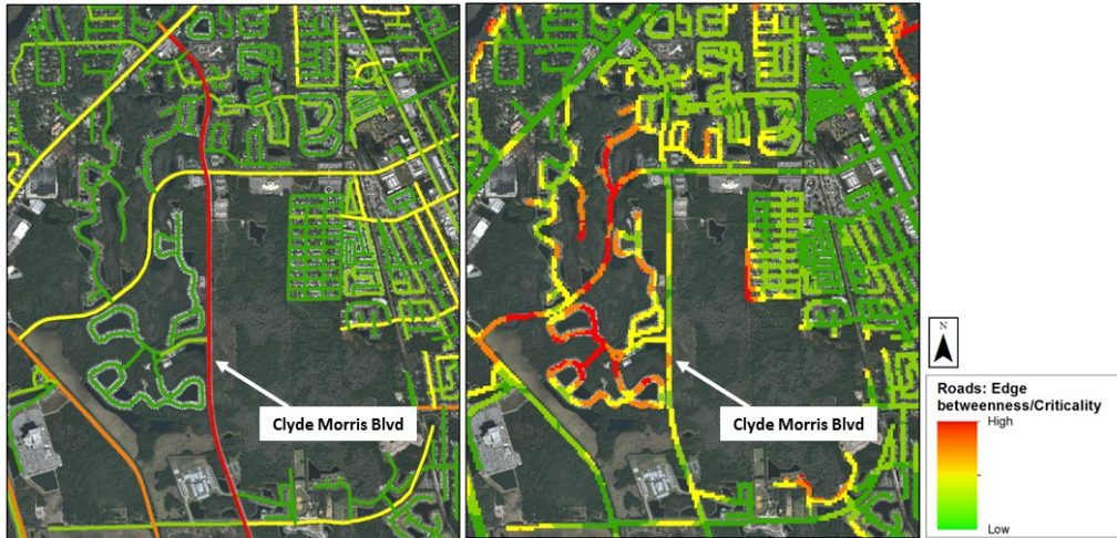
Figure 5.3. Traditional edge betweenness centrality scores (5.3a) and the grid-based criticality measurements (5.3b). Note the differences along Clyde Morris Boulevard, the lengthy north-south thoroughfare running through the figure.
