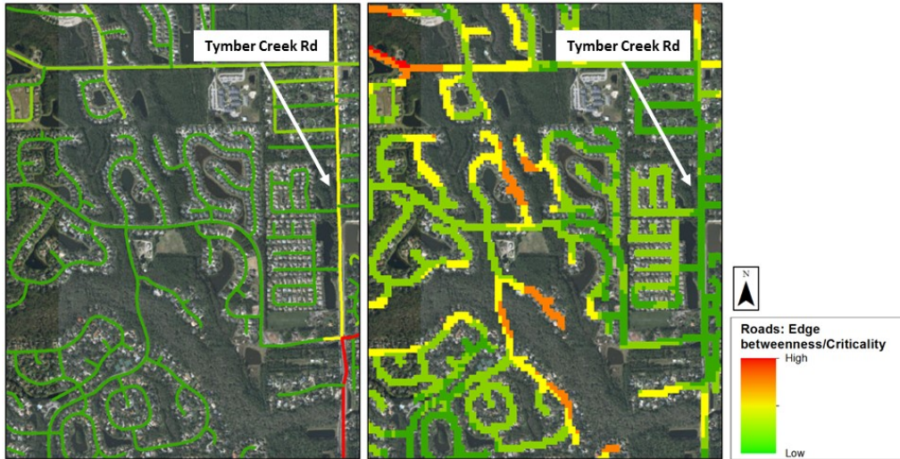
Figure 5.5. Traditional (5.5a) and modified (5.5b) criticality measurements for residential areas in western Ormond Beach, Florida. Traditional edge betweenness metrics identify these roads as non-critical, but due to the relative impassability of the surrounding terrain, they receive elevated criticality scores from the modified grid-based approach.
