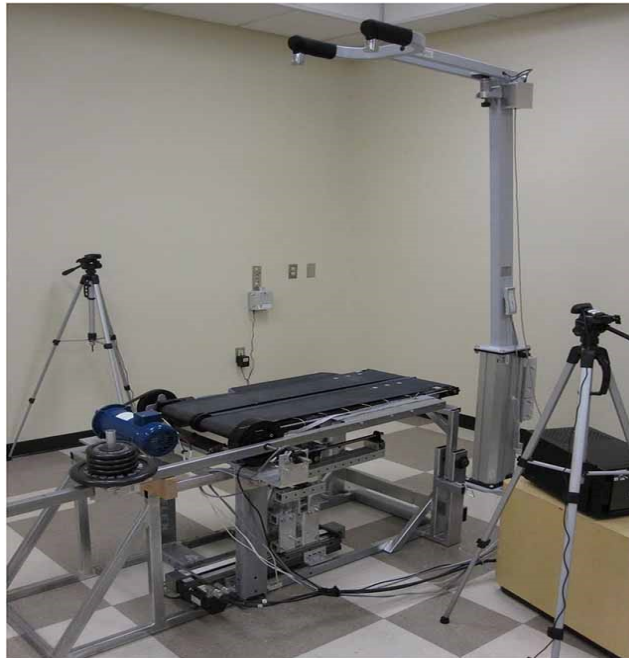
Figure 3.4: The Variable Stiffness Treadmill Developed by Skidmore, Barkan and Artemiadis
