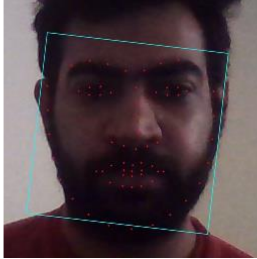
Figure 14: Using facial landmarks to perform face alignment step
